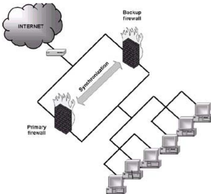
Fig. 2.29: Scheme of a cluster comprising two firewalls
