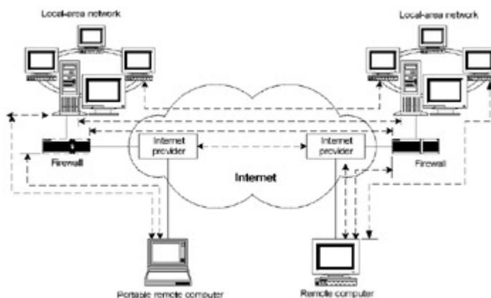
Fig. 3.3: Versions of protected virtual channels
