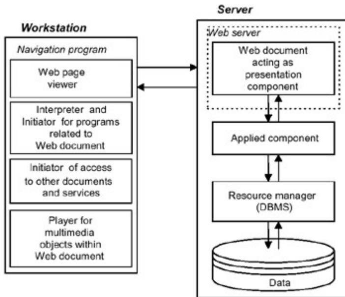
Fig. 1.8: Client/server architecture based on Web technology
