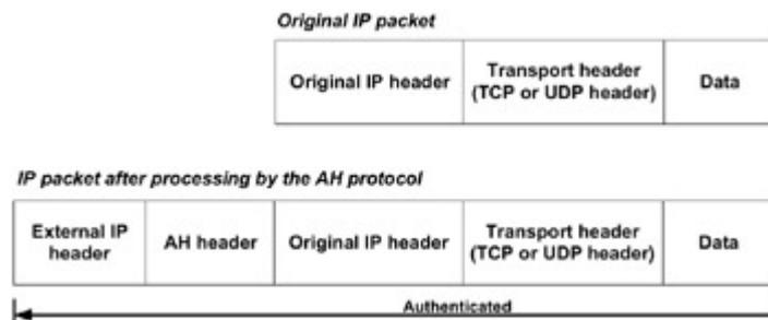
Fig. 3.9: The IP packet before and after processing by an AH protocol in tunnel mode
