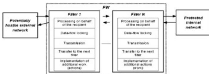
Fig. 2.11: Structure of the firewall
