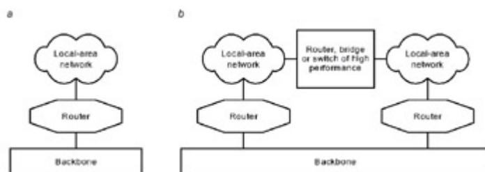
Fig. 1.41: Connection to a backbone
