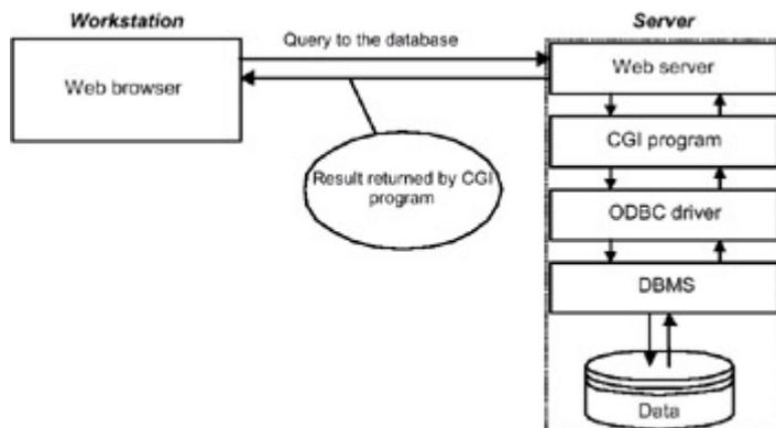
Fig. 1.16: Access to DBMS through CGI program
