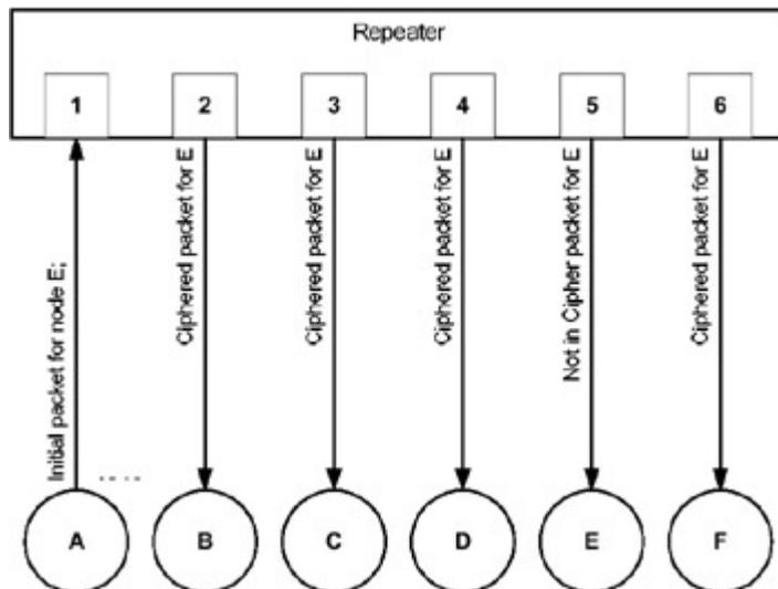
Fig. 1.30: The transmission of a packet from computer A to computer E
