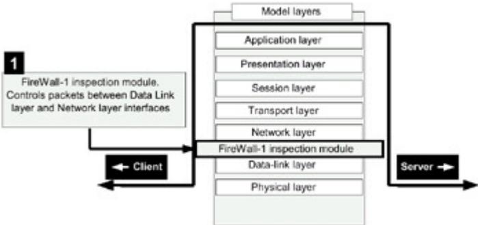
Fig. 2.24: The scheme of inspection-module operation
