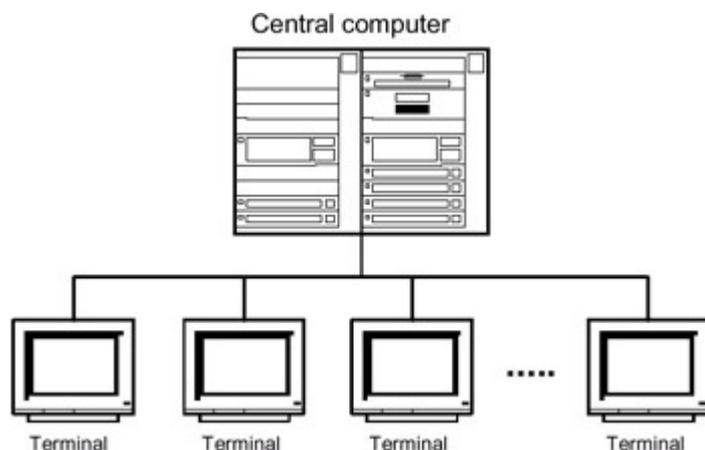
Fig. 1.2: The architecture of the first computing systems
