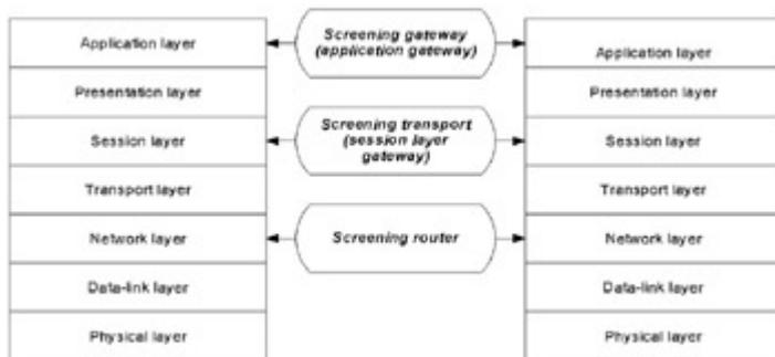
Fig. 2.12: Types of firewalls operating at separate layers of the OSI model
