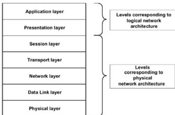
Fig. 1.1: The relationship between standard OSI layers and types of network architecture
