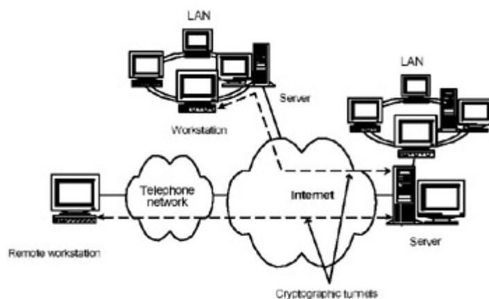
Fig. 3.14: Cryptographic tunnels based on the SSL protocol
