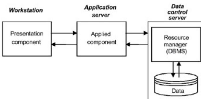
Fig. 1.7: Three-tier client/server architecture
