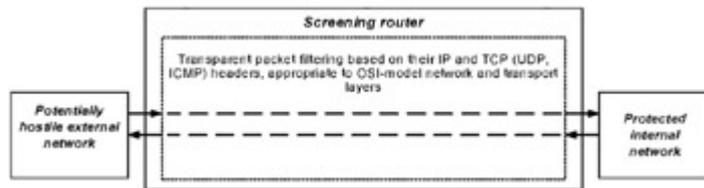
Fig. 2.13. The operation scheme of a packet filter
