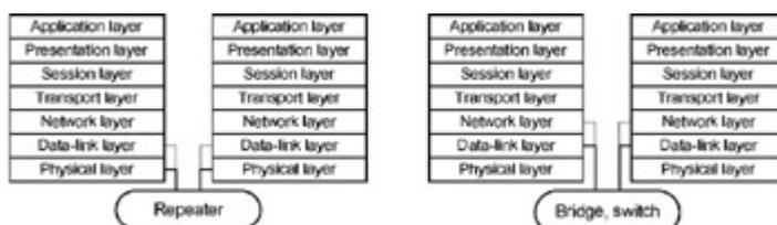
Fig. 1.27: The layers of the OSI model with repeaters and bridges
