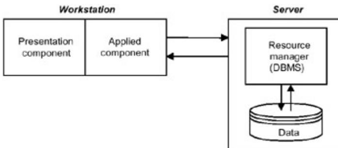
Fig. 1.5: Data control server model
