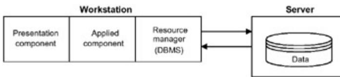
Fig. 1.4: Model of access to remote data
