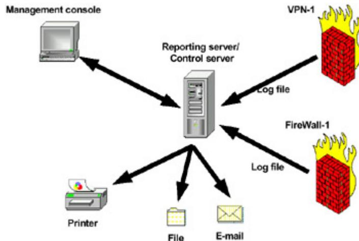
Fig. 2.27: The scheme of Reporting Module usage
