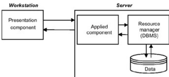
Fig. 1.6: Two-tier client/server model
