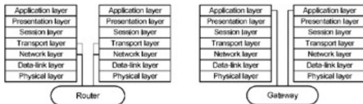
Fig. 1.28: The layers of the OSI model with routers and gateways
