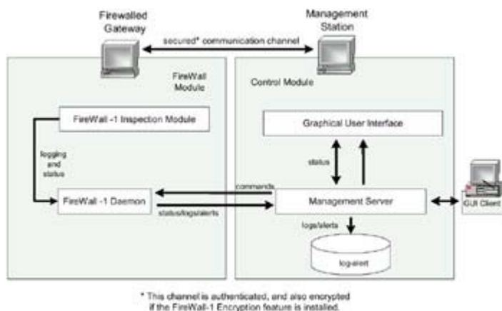
Fig. 2.23: Scheme of interaction between FireWall-1 components
