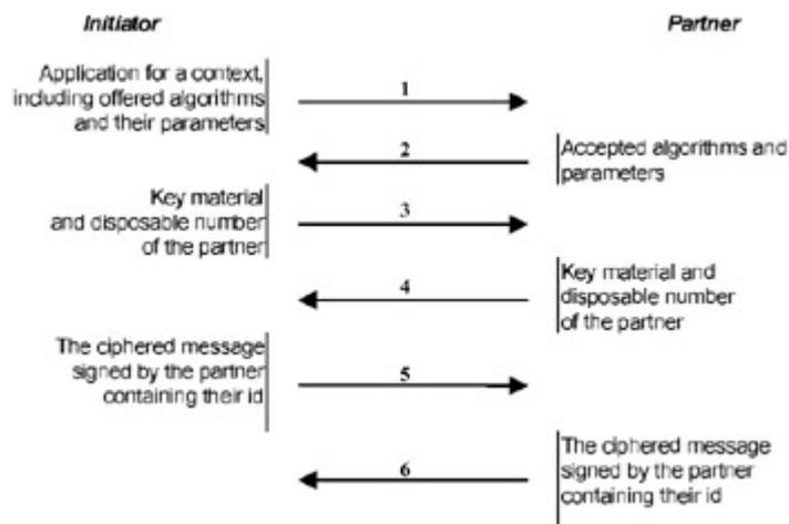
Fig. 3.17: The scheme of coordination of global parameters of a protected channel
