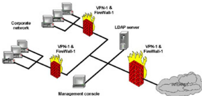
Fig. 2.26: The scheme of LDAP Account Management Module usage
