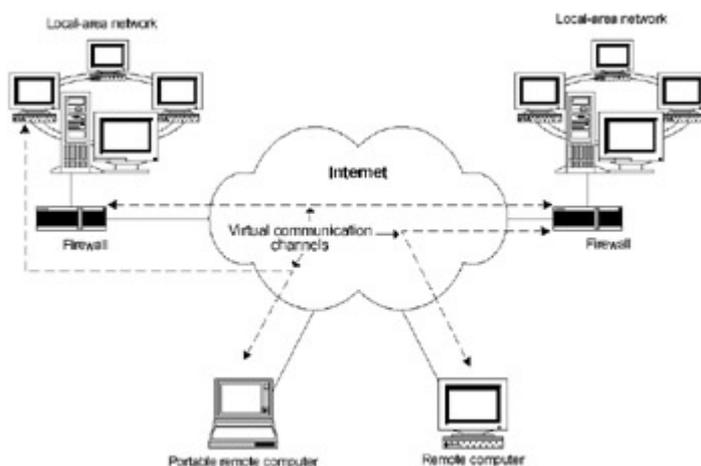
Fig. 3.2: Construction of a virtual network on the basis of the Internet.
