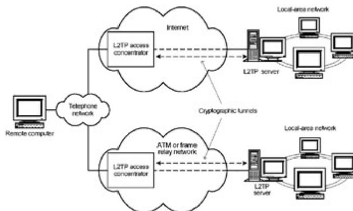
Fig. 3.7: Interaction scheme under the L2TP protocol
