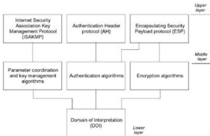
Fig. 3.8: The IPsec architecture
