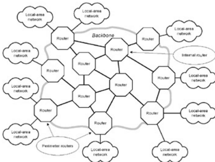
Fig. 1.43: A backbone as a routed cloud
