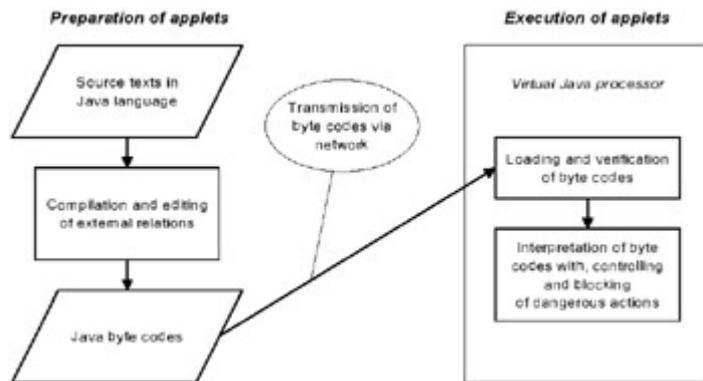
Fig. 1.13: Preparation and execution of Java applets
