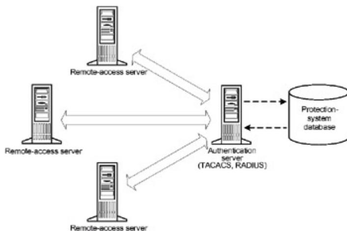
Fig. 3.26: Centralized remote-access control
