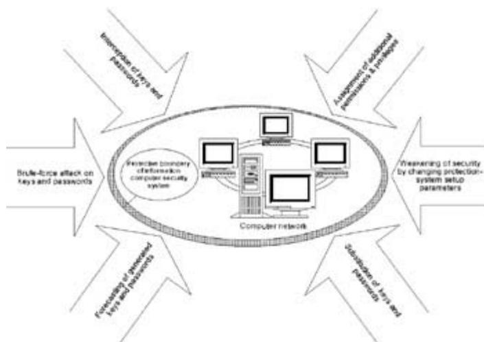
Fig. 2.7: Attacks on changeable components of a security system
