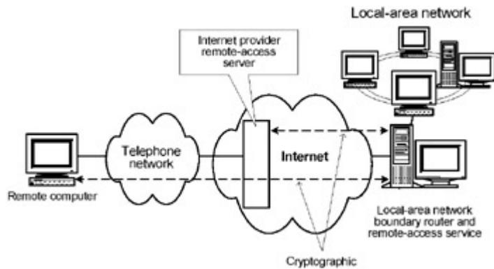
Fig. 3.5: Tunneling scheme upon connection of a remote computer to the Internet through a provider using a telephone line
