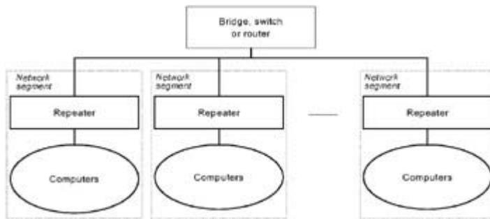
Fig. 1.29: The connection of network segments
