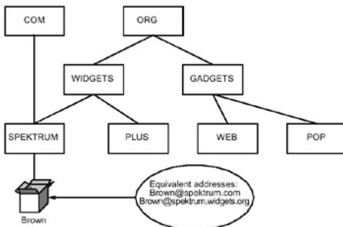
Fig. 1.26: An example of a hierarchical diagram of addressing in SMTP
