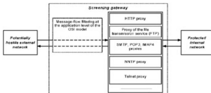
Fig. 2.16: The operation of an application gateway
