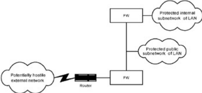
Fig. 2.21: A scheme with separate protection of internal and public subnets on the basis of two firewalls with two network interfaces
