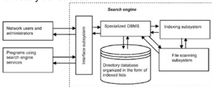
Fig. 1.22: The usage and organization of a search engine, based on the construction of indexes
