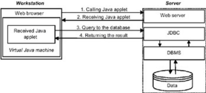
Fig. 1.17: Access to a DBMS with the help of a Java applet
