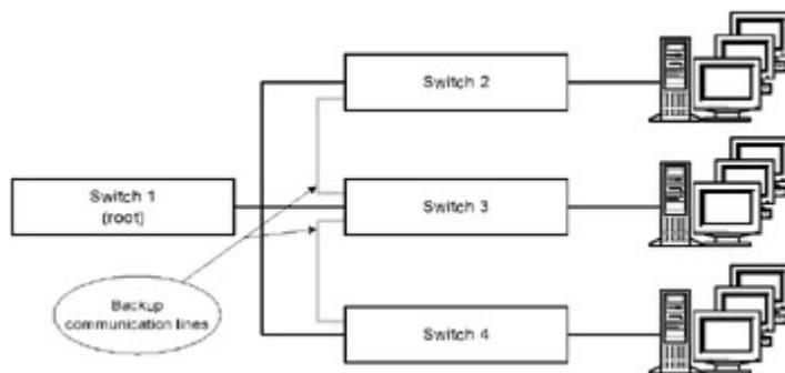
Fig. 1.36: Construction of a local-area network through a hierarchy of switches with backup communication lines
