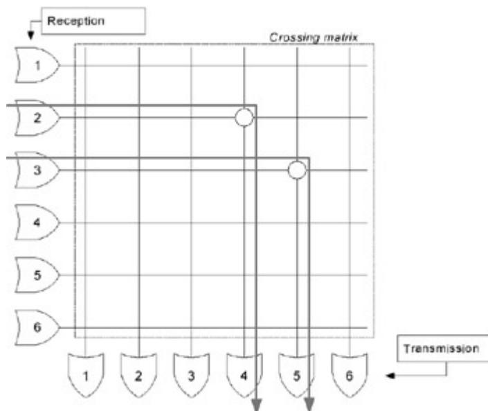
Fig. 1.34: The logical scheme of a switch
