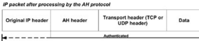
Fig. 3.10: The IP packet before and after processing by the AH protocol in transport mode
