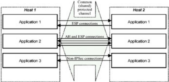
Fig. 3.19: Protected interaction under the ISAKMP protocol
