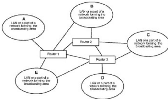
Fig. 1.38: Interconnection of broadcasting areas with the help of routers
