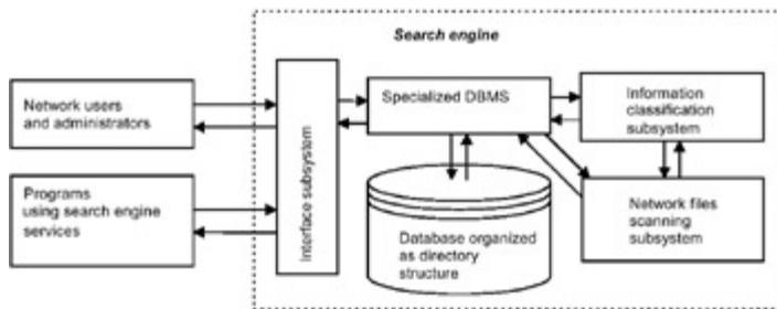
Fig. 1.21: The usage and organization of an information-retrieval system based on directory construction
