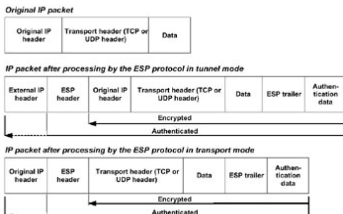
Fig. 3.13: The IP packet before and after applying the ESP protocol
