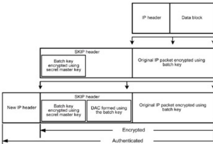
Fig. 3.16: IP packet before and after use of the SKIP protocol
