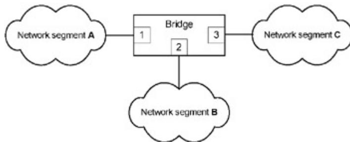
Fig. 1.31: The connection of segments of a local-area network with a bridge
