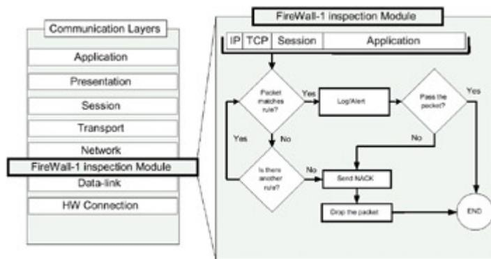
Fig. 2.25: Architecture of the inspection module
