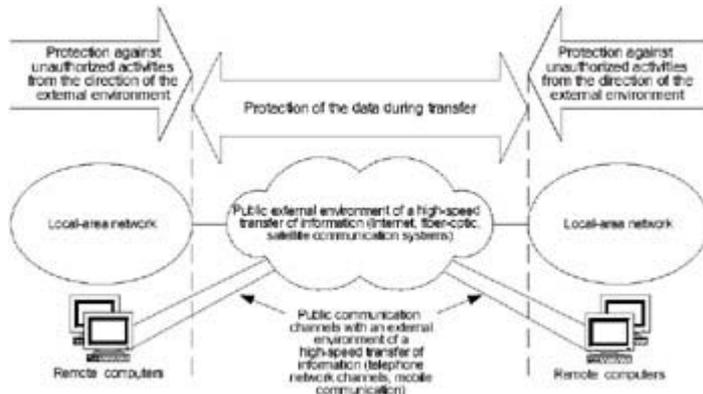
Fig. 3.1: Tasks of providing security of information interaction
