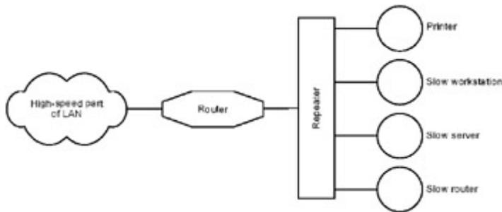
Fig. 1.40: The protection scheme for slow devices against overloading
