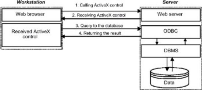
Fig. 1.18: Access to a DBMS with the help of an ActiveX control
