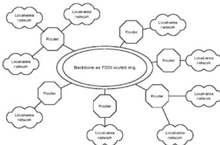
Fig. 1.42: A backbone as a routed ring
