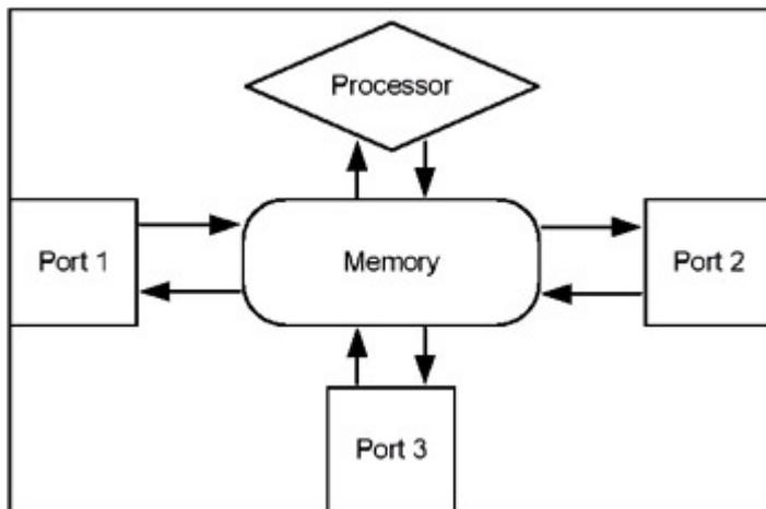
Fig. 1.32: The simplified architecture of a bridge with three ports
