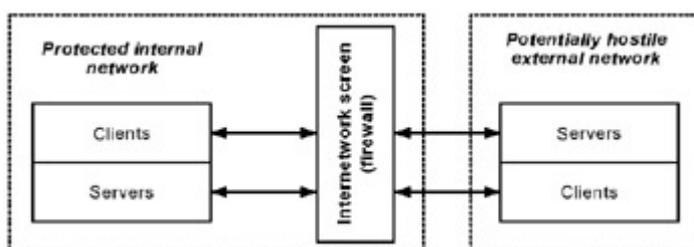
Fig. 2.10: The connection scheme of an internetwork screen (firewall)
