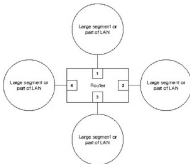
Fig. 1.39: The interconnection of parts of a large network
