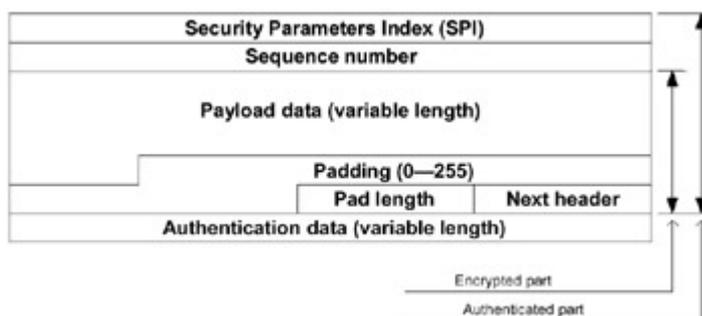
Fig. 3.12: The ESP packet header
