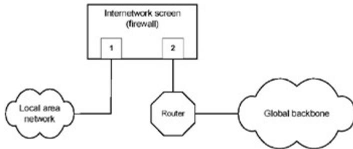
Fig. 1.44: Secure connection to a global network
