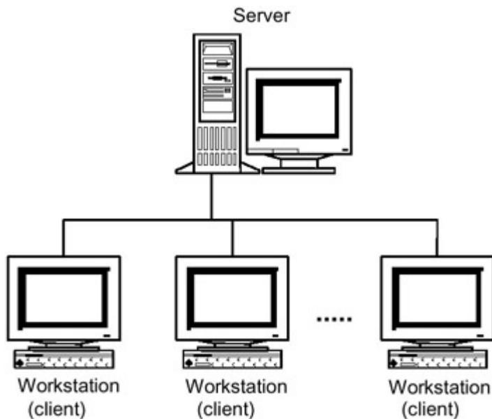
Fig. 1.3: Standard client/server architecture
