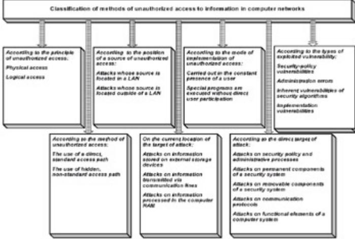
Fig. 2.1: Classification of methods of attacks on computer networks
