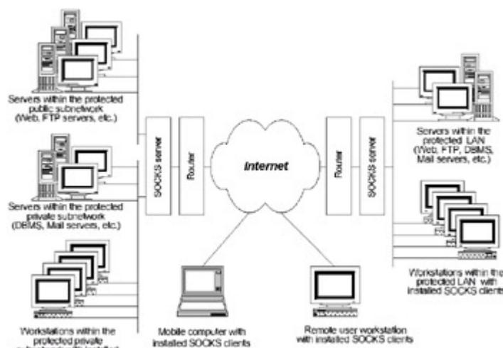
Fig. 3.15: The scheme of network interaction under the SOCKS protocol
