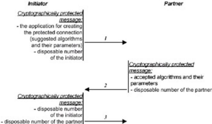
Fig. 3.20: The scheme of parameters of two symmetric connections
