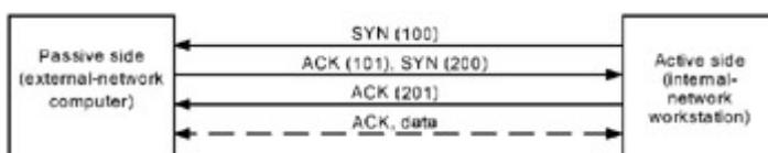
Fig. 2.14: The scheme of acknowledgement of connection by the TCP protocol
