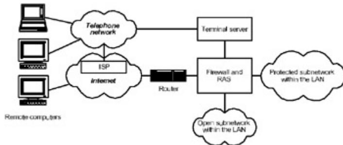
Fig. 3.22: Secure configuration of the LAN when organizing remote access
