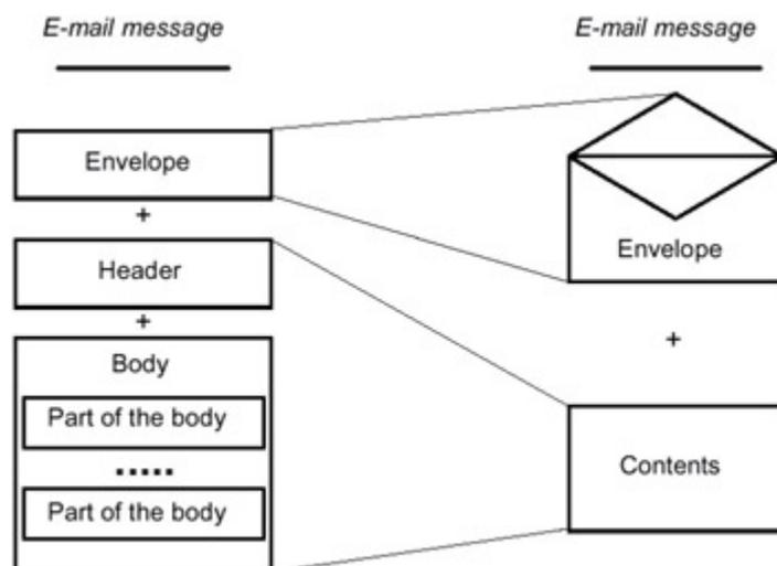
Fig. 1.24: The electronic message's structure
