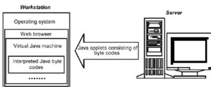
Fig. 1.12: The transfer and execution of machine-independent Java programs
