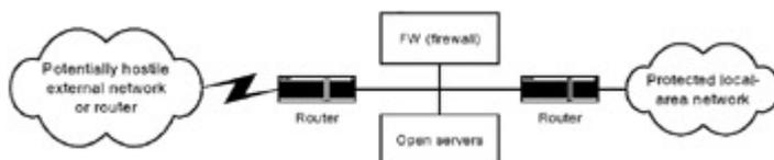
Fig. 2.17: Protection of a local-area network with a firewall with one network interface
