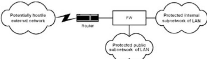
Fig. 2.20: A scheme with separate protection of internal and public subnets on the basis of one firewall with three network interfaces
