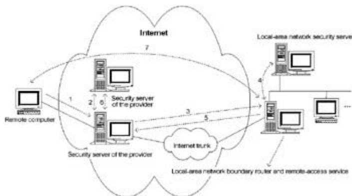
Fig. 3.6: Interaction scheme under the L2F protocol
