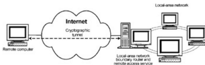
Fig. 3.4: The tunneling scheme at direct connection of a remote computer to the Internet
