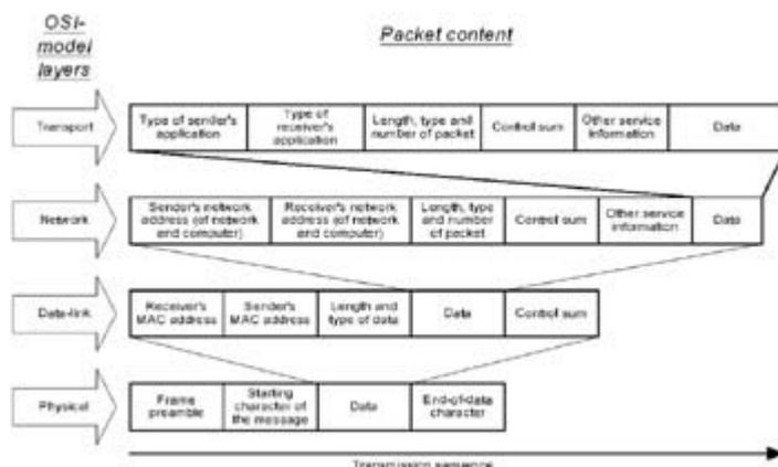
Fig. 1.37: The scheme of encapsulation of a transmitted packet
