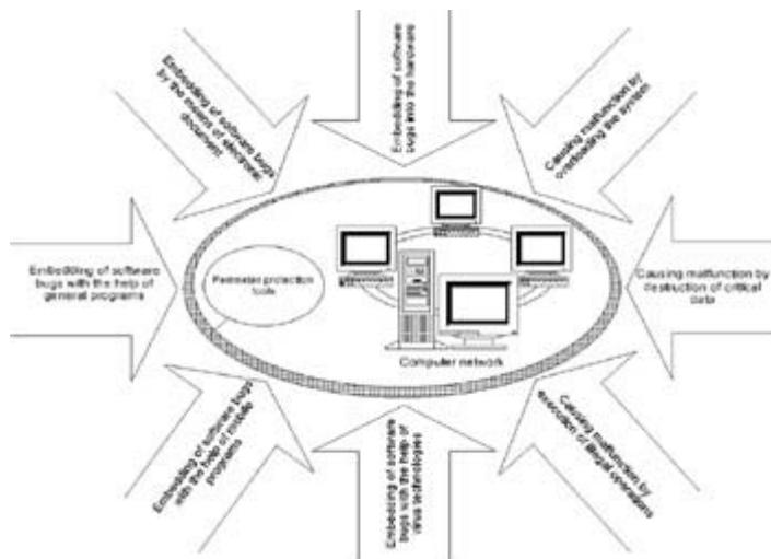
Fig. 2.9: Attacks on functional elements of computer networks
