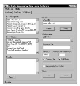
**Figure 11-4:** WebBrute allows you to scan your Web directories that are protected with HTTP authentication, testing the security strength of your users' passwords.
