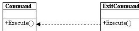
Figure 2.4 – ExitCommand implements the Command interface.
