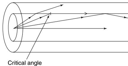
**Figure 2-9** Total internal reflection in an optical fiber.
