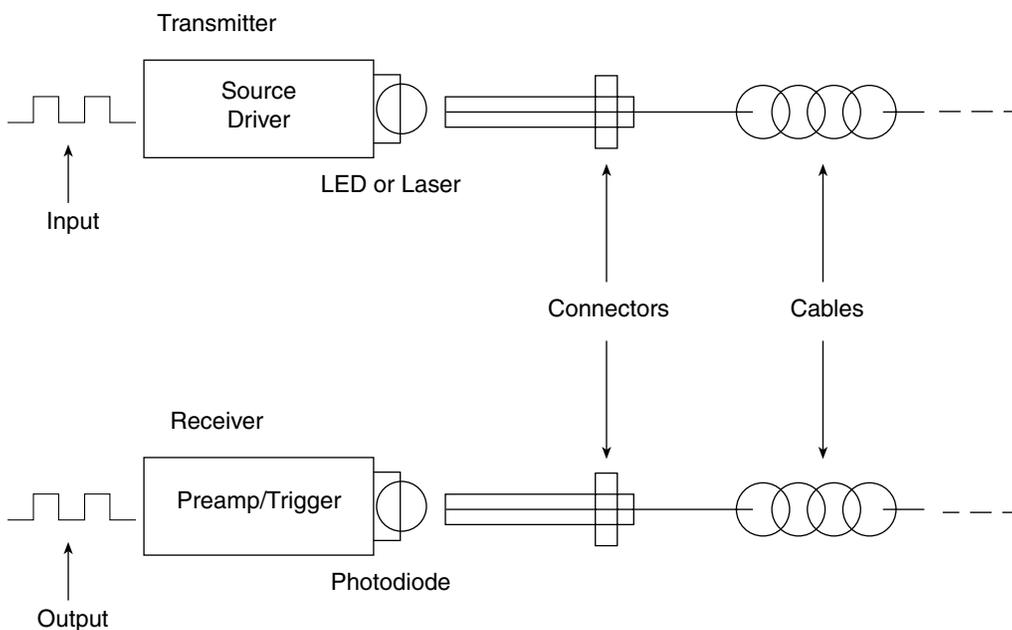
**Figure 2-1** A typical fiber optic data link.
