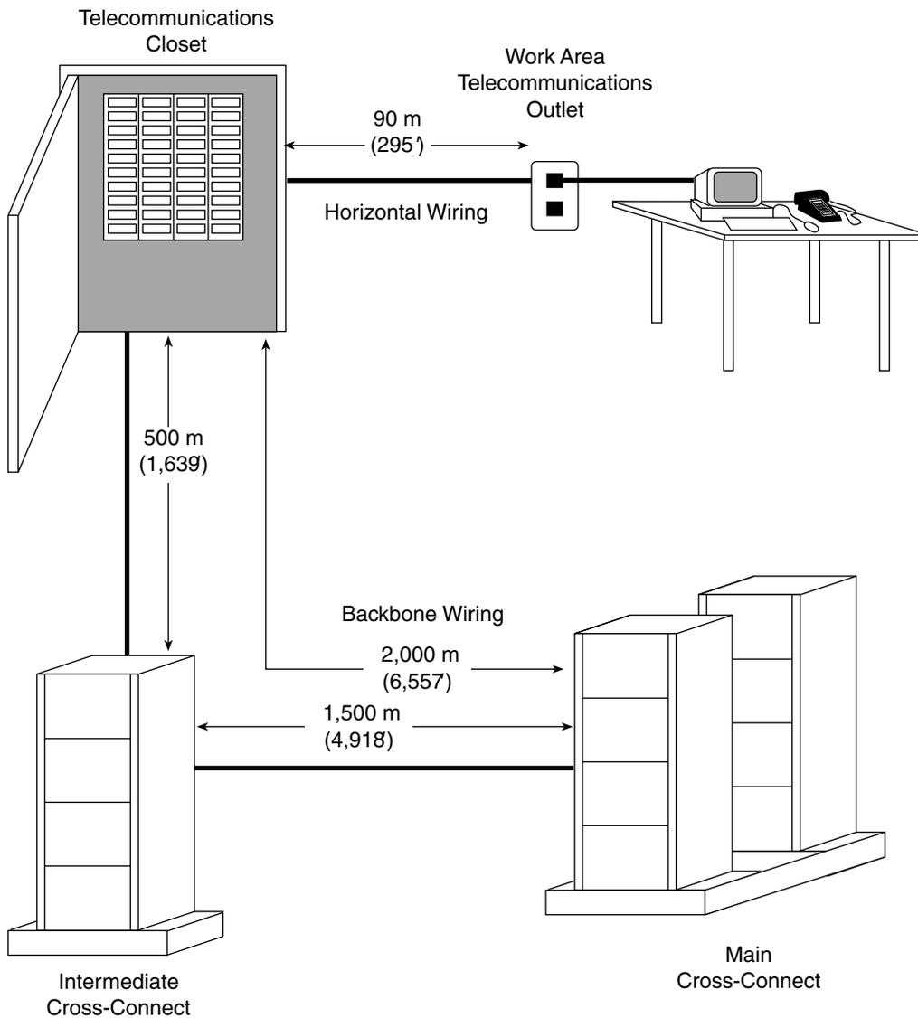
**Figure 7-1** Backbone cabling.
