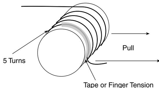
**Figure 15-6** Using a mandrel for pulling cable.
