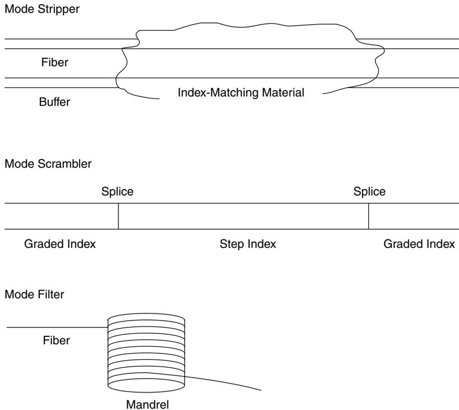
**Figure 17-9** Mode conditioners for multimode graded-index fibers.
