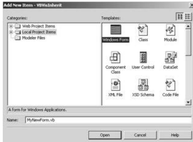
Figure 9.12: The Add New Item dialog lets you create a new form and add it to a project.
