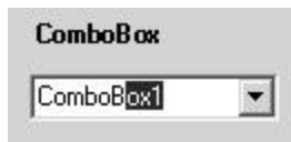
Figure 10.7: A ComboBox with DropDown style showing the list hidden and text selected in the edit control.
