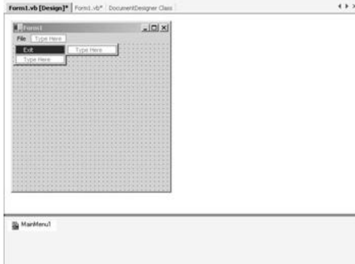
Figure 9.14: Creating a menu in a Windows Forms application.
