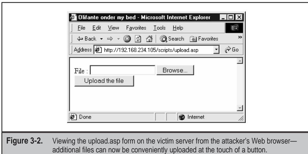
**Figure 3-2.** Viewing the upload.asp form on the victim server from the attacker's Web browser—additional files can now be conveniently uploaded at the touch of a button.
