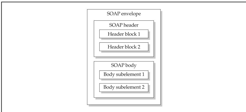
**Figure 10-2.** A schematic representation of a SOAP message, showing envelope, body, and headers
