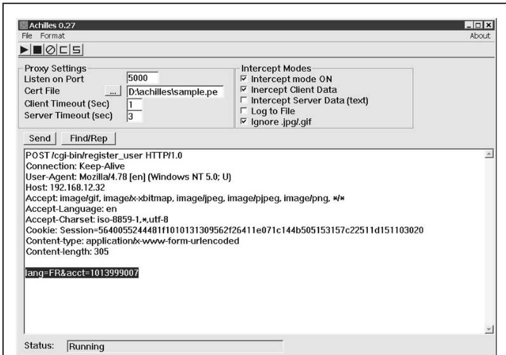
**Figure 8-1.** Using Achilles to bypass input validation routines
