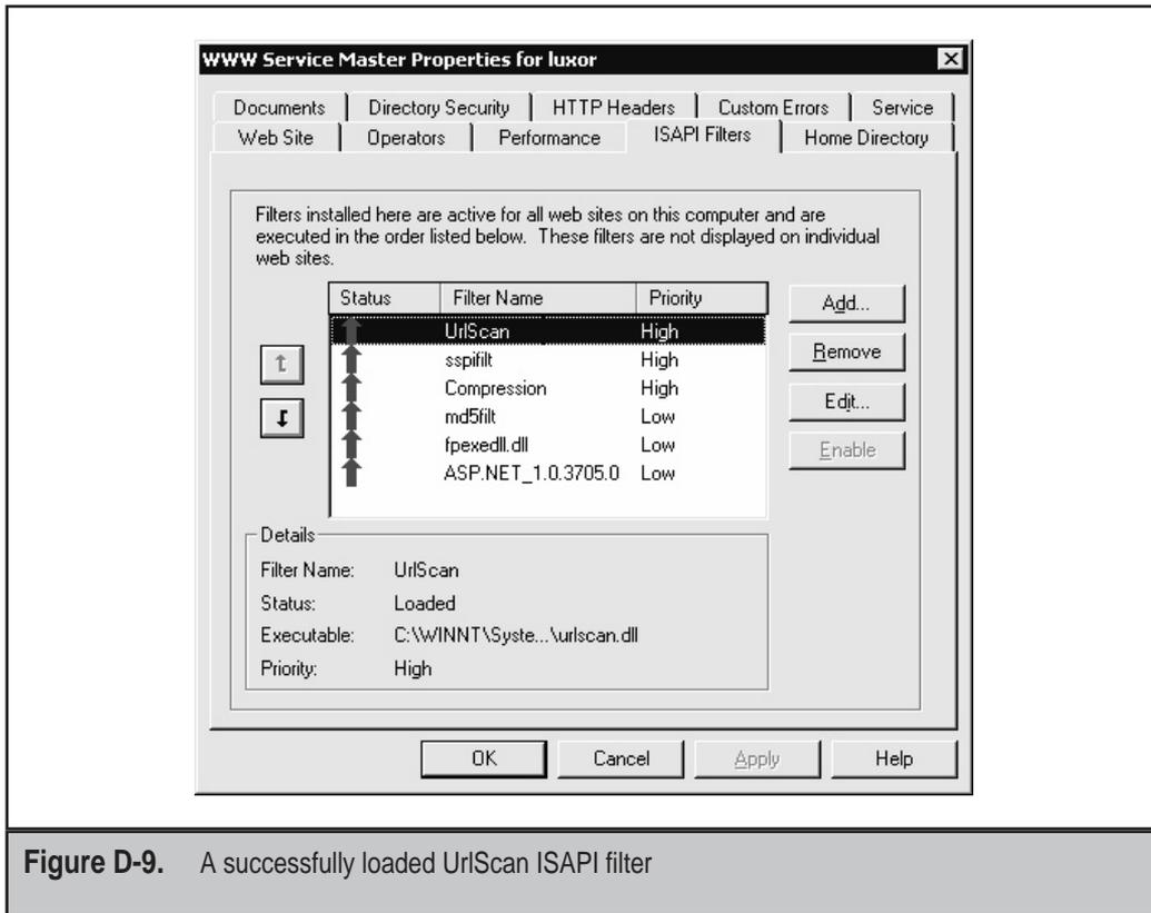
**Figure D-9.** A successfully loaded UrlScan ISAPI filter
