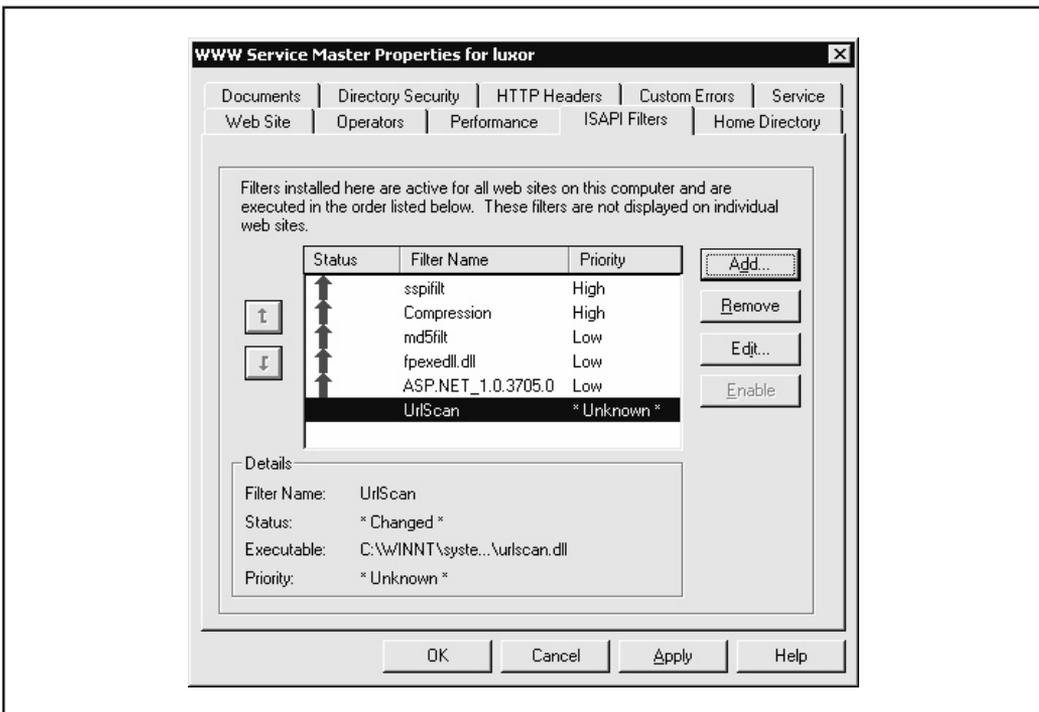
**Figure D-8.** Immediately after installing the UrlScan ISAPI filter, it is left in an Unknown state.
