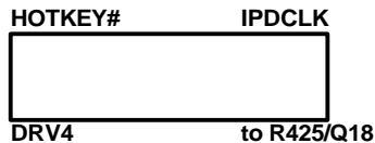
Keyboard Connector Top View
