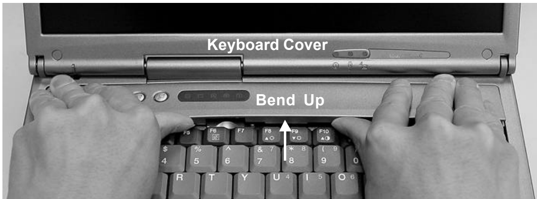
Figure 5-2 Remove keyboard cover
