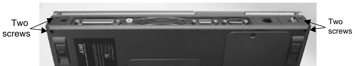
Figure 5-9 Four Screws Securing the LCD Hinges
