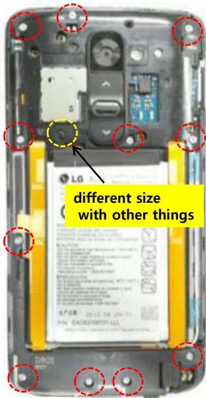
1) Disassemble the Rear, SPK module Screws. (Screw Point : 12Point)
