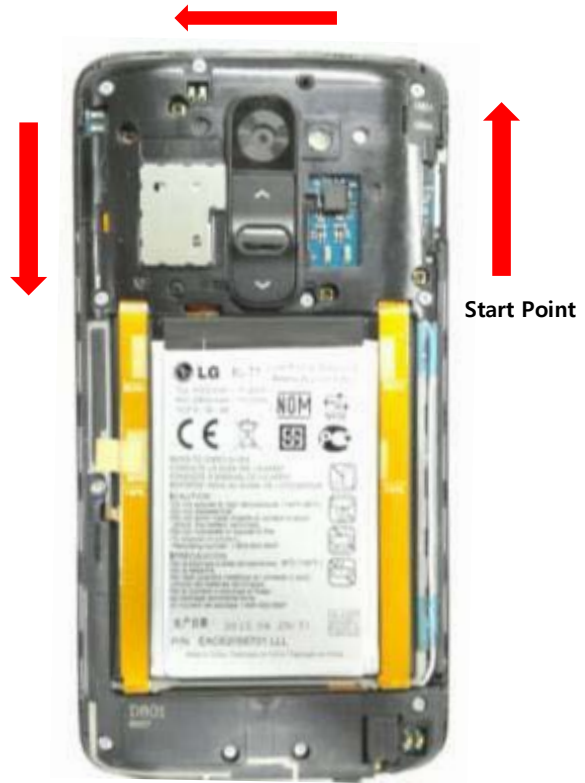
2) Unhook Rear cover along below direction.
