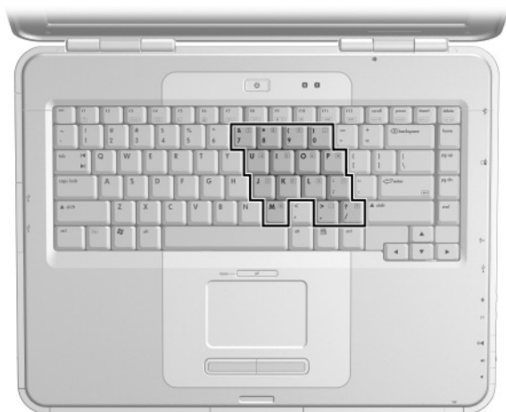
Identifying the keypad keys
