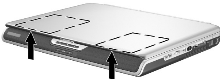
Identifying the wireless antenna
