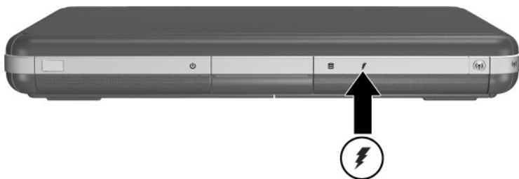
Identifying the battery light
