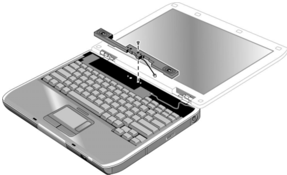
Figure 2-11. Removing the Speaker Assembly
