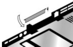
Figure 2-37. Removing a PCMCIA Door
