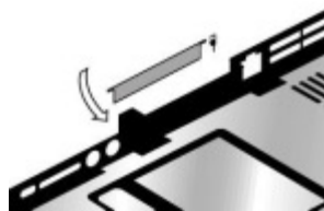
Figure 2-37. Removing a PCMCIA Door
