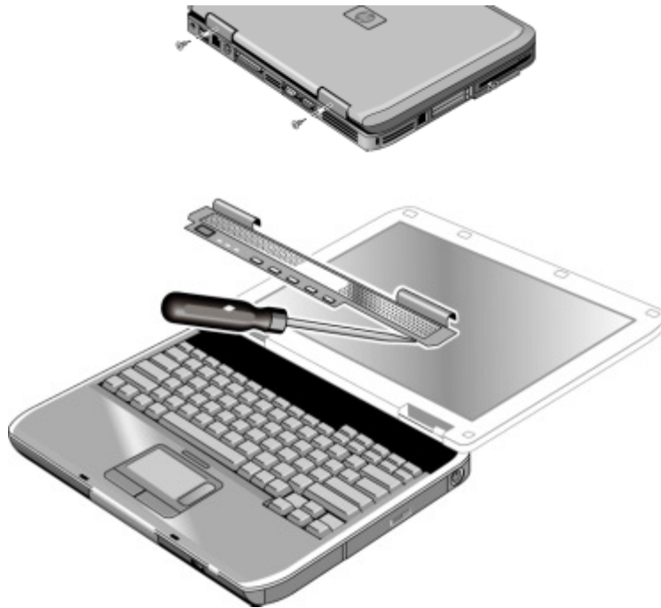
Figure 2-9. Removing the Keyboard Cover
