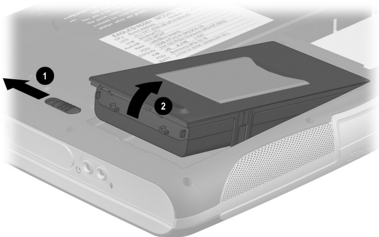
Figure 5-2. Releasing the Battery Pack
