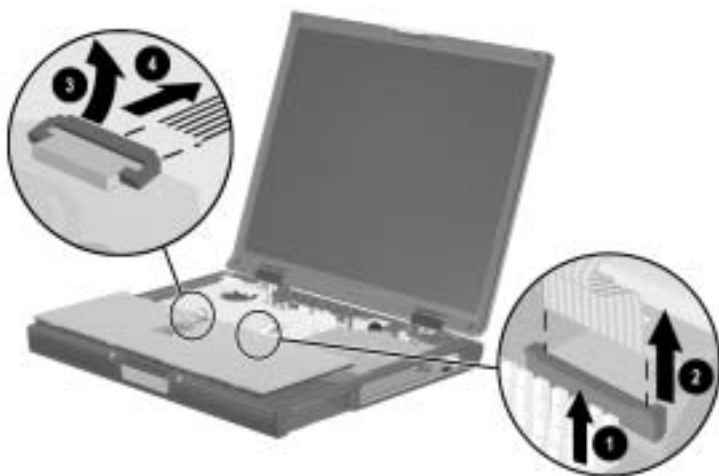
Figure 5-19. Disconnecting the Keyboard-to-TouchPad Cable
