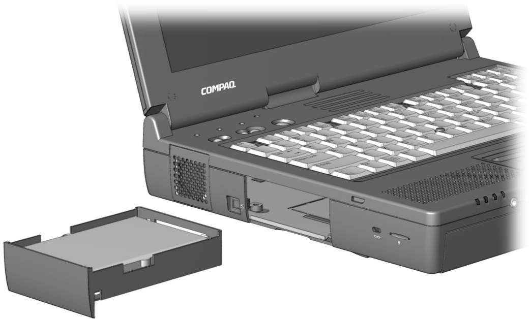
Figure 5-16. Inserting a Hard Drive into the Hard Drive Bay
