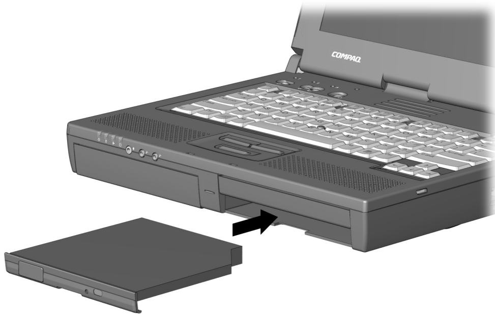
Figure 5-21. Inserting a Device into a MultiBay
