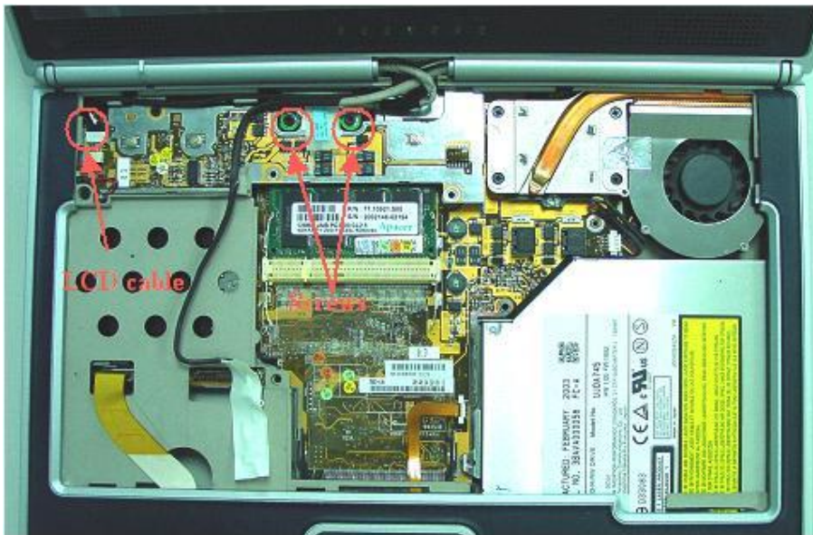
Figure 5-10 Two Screws and one LCD cable
