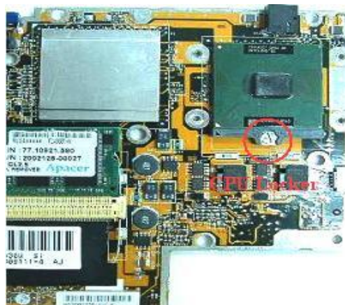
Figure 5-12 CPU Assembly
