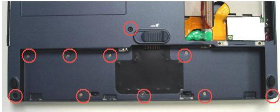
Figure 5-14 Removing the eleven screws of bottom case
