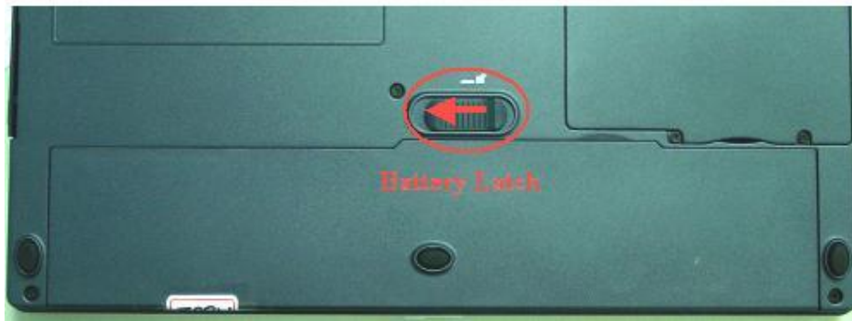
Figure 5-2 Removing the battery pack
