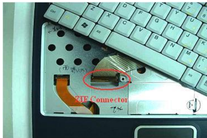
Figure 5-5 Remove keyboard
