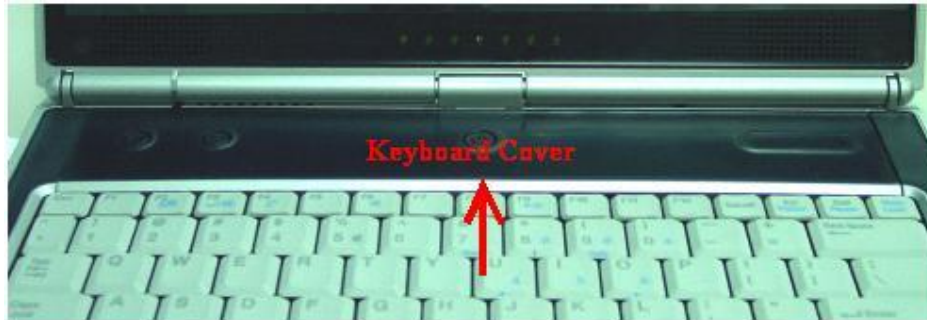
Figure 5-4 Remove Keyboard Cover
