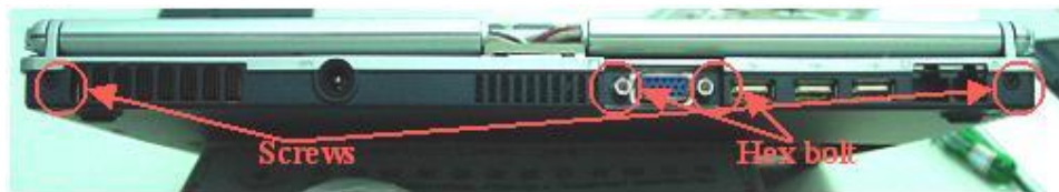
Figure 5-9 Two Screws and two hex-bolds
