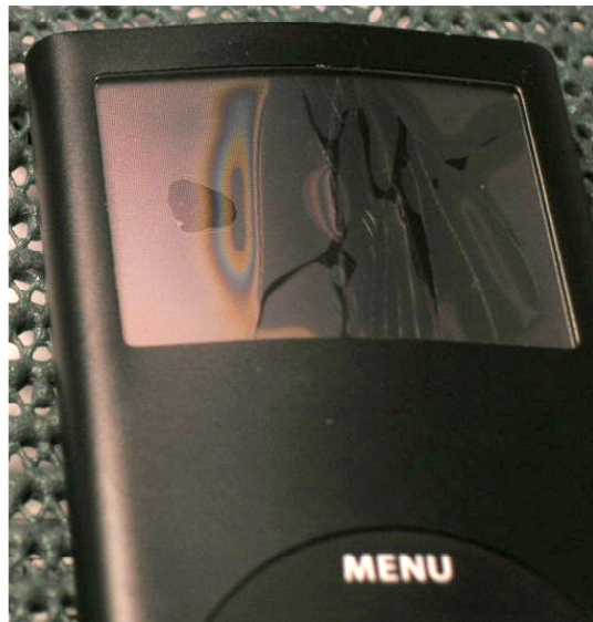
Bent case and cracked LCD due to battery swelling — COVERED
