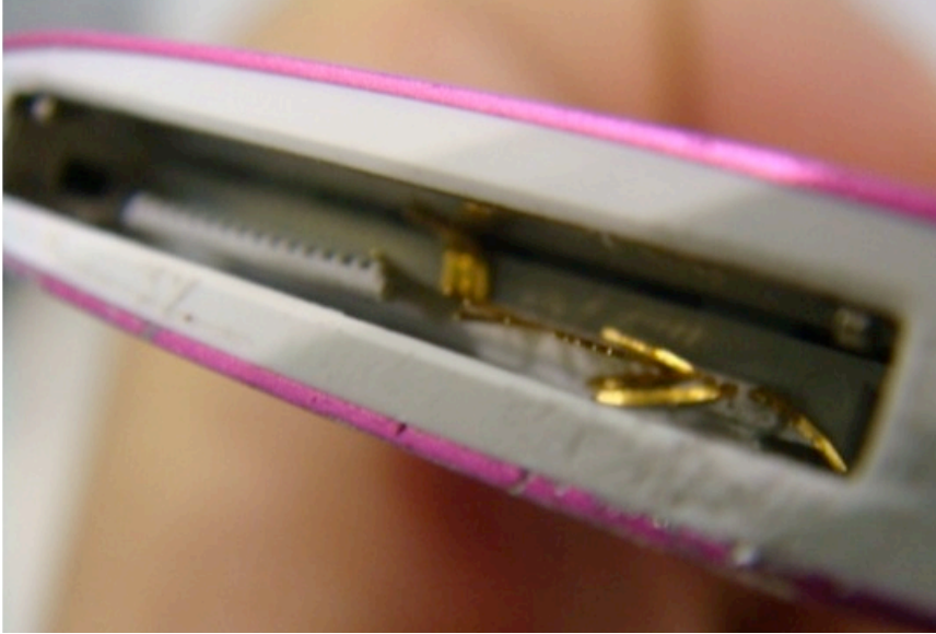
Dented housing — Failure NOT Covered
