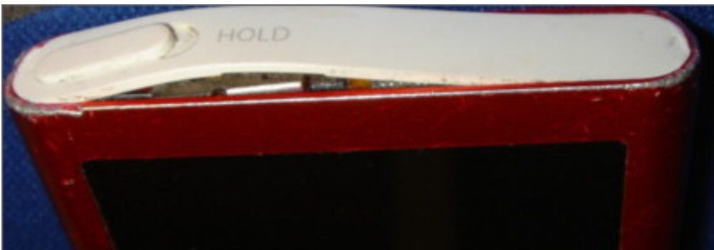
Deformed edge causing plastic cover to warp — Failure NOT Covered
