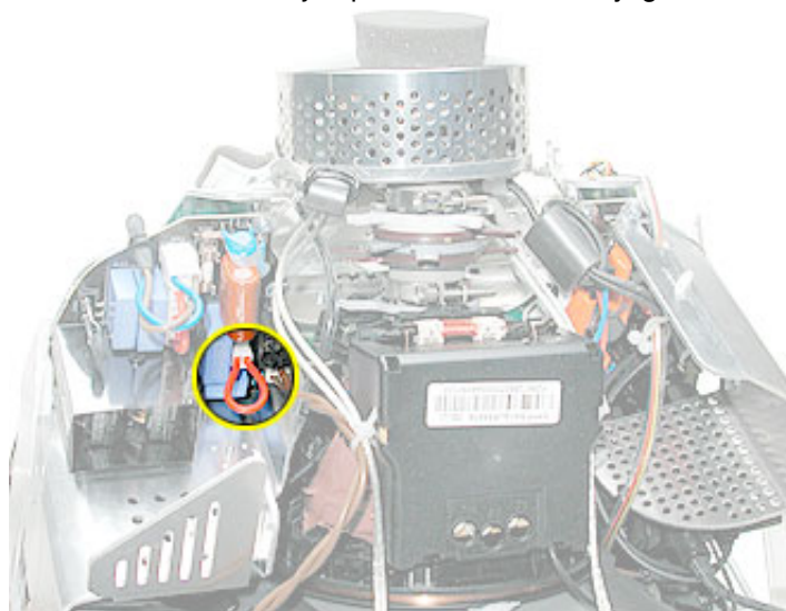
Voltage Jumper Location
