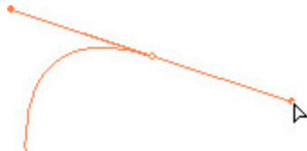
Figure 4.9: The resulting curve that is created as you move the selected tangent handle away from the original end point. Note that the tangent handle stretches out the farther you drag it away.
