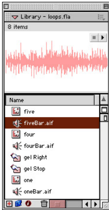
Figure 20.1: The Library panel displays sound files with a speaker icon beside the filenames.
