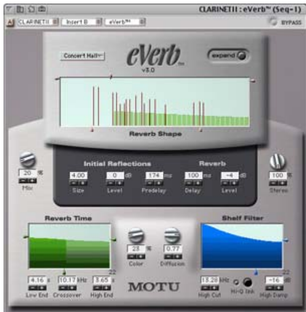
Figure 25.8: Digital Performer's eVerb plug-in has many options for fine-tuning the reverb setting parameters
