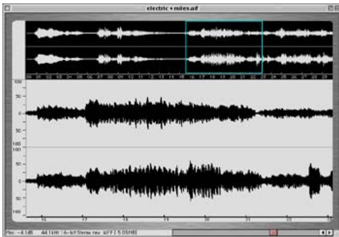
Figure 25.4: The Peak interface provides two levels of navigation for a sound file, regular (detailed waveform) and Overview, shown in the topmost window.
