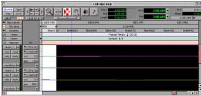
Figure 25.11: When making your loop selection, be sure that the selection begins at a point in the sound wave (or waves, if stereo) where there is a zero crossing.
