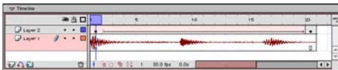
Figure 21.3: In this Timeline, the stream sound that starts at frame 1 is stopped to sync with an event in the animation at frame 20.
