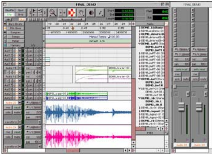
Figure 25.1: Pro Tools LE has all the editing features of regular Pro Tools but depends on the host computer to do any digital signal processing (DSP).
