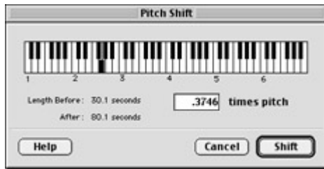
Figure 25.9: The Pitch Shift window in SoundEdit 16 uses a keyboard graphic to set changes in pitch based on the intervals of a keyboard.
