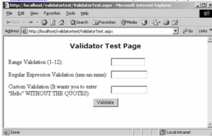
Figure 5-7 : ValidatorTest.aspx, which uses the RangeValidator , RegularExpressionValidator , and CustomValidator controls
