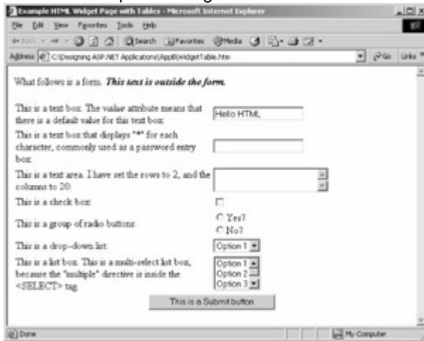
Figure B-2 : The results of displaying the HTML from Listing B-2 in Internet Explorer, using a table to format the form
