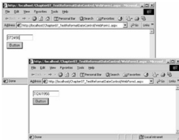
Figure 7-4 : The ReformatDate control, before and after tabbing out of it Listing 7-7 shows the code for the completed ReformatDate control.
