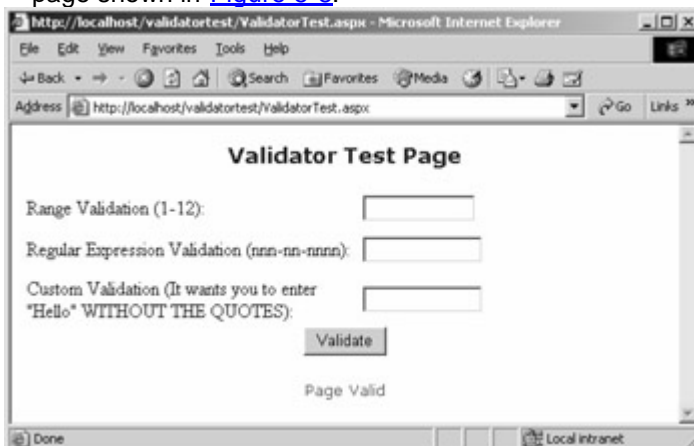
Figure 5-8 : The page that results from clicking the Validate button with no values filled in. Notice that it displays the message "Page Valid". This is almost certainly not what you wanted! You specified that the first field should be a number between 1 and 12, that the
