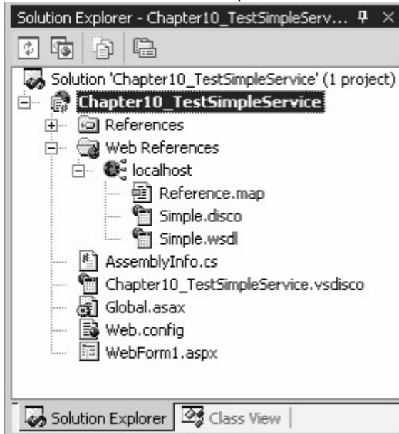
Figure 10-6 : Solution Explorer, showing the newly added Web reference to the Simple service
