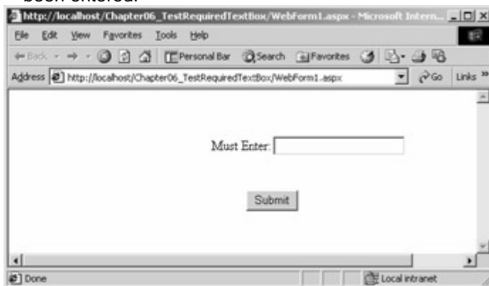
Figure 6-8 : The test page for the RequiredTextBox custom control
