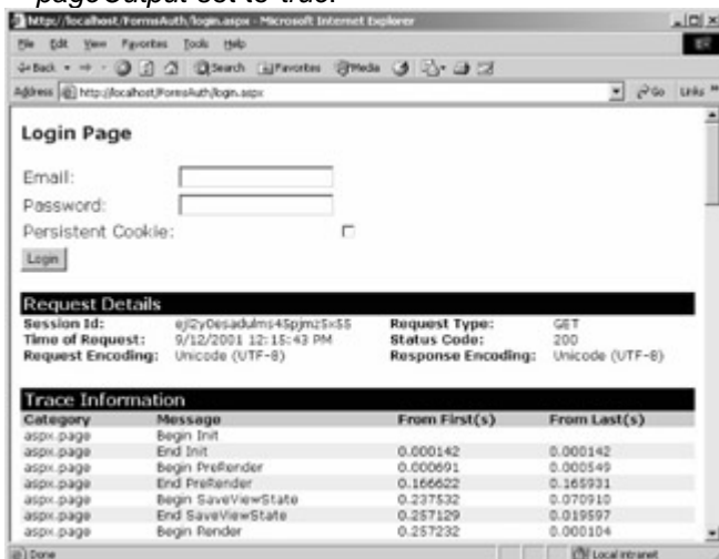
Figure 4-15 : The output of the Login.aspx page shown in Listing 4-6 when tracing is enabled and pageOutput is set to true
