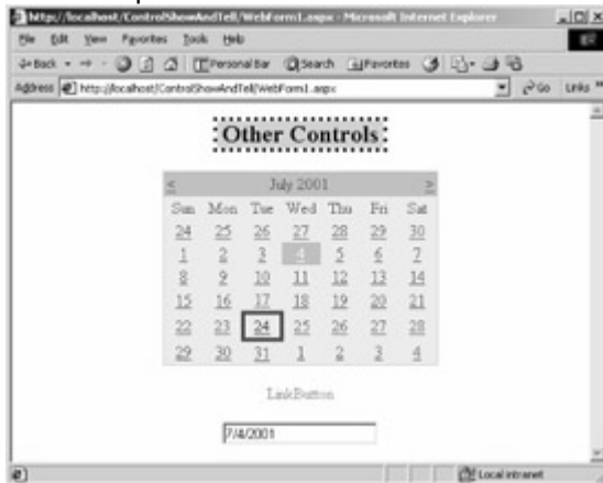
Figure 5-12 : WebForm1.aspx , showing Today'sDate as set in code, with July 4 as the selected date
