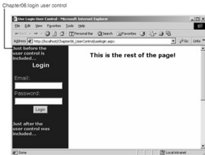
Figure 6-3 : The page created by running UseLogin.aspx as shown in Listing 6-3 . The user control appears to integrate seamlessly within the page. The login section can be included in many pages. Although this was possible using server-side include files in ASP, user controls offer the advantage of compiled code. Listing 6-4 shows the HTML sent to the browser when UseLogin.aspx is requested.
