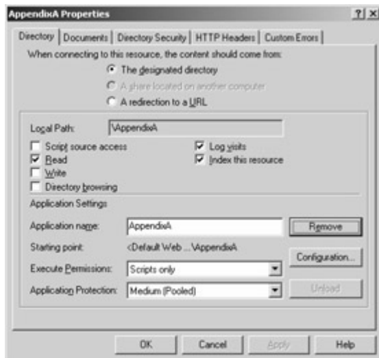
Figure A-3 : The Properties dialog box in Internet Information Services for the AppendixA folder after it has been made a virtual directory
