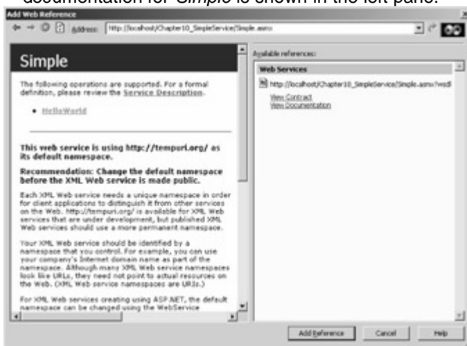
Figure 10-5 : The Add Web Reference dialog box in Visual Studio .NET, pointing to the Simple XML Web service
