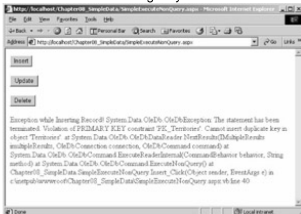
Figure 8-4: The exception information displayed by SimpleExecuteNonQuery.aspx when you insert a record that already exists
