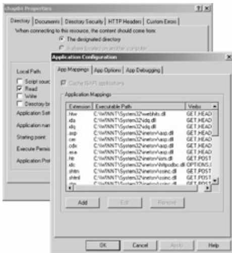
Figure 4-7 : Application Configuration dialog box for newly created chap04 application directory
