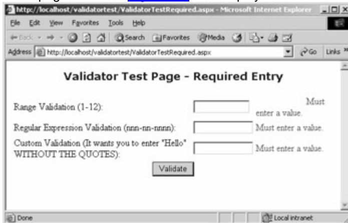
Figure 5-9 : The result when the first validator on a given field is set to Static display. The ErrorMessage associated with the first validator (which hasn't been fired) is "Out of Range". Looking at Figure 5-9 , you can see that the space between the text box and the beginning of the first "Must enter a value" string is about what might be required to fit "Out of Range". Because we have the actual source that generated this page, we can see what the browser uses to render the page. The following HTML code is the table row returned to the browser in which the range validator is located. (The code has been reformatted for readability.)
