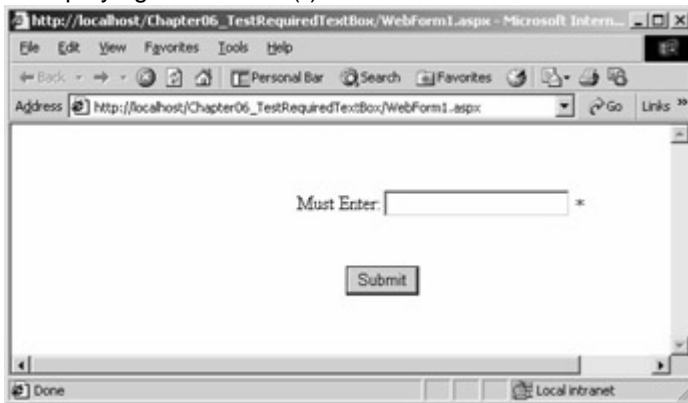
Figure 6-9 : The test page for RequiredTextBox after the page is submitted with a blank field. The validation that has taken place in Figure 6-9 is on the client. Add a ClientTarget=Downlevel attribute/value pair to the @ Page directive and each click of the submit button will require a round-trip to the server.
