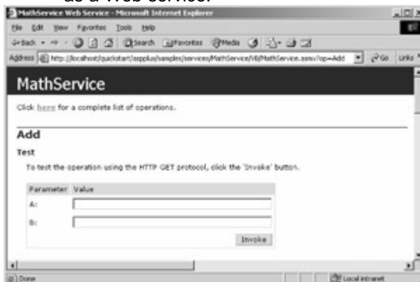
Figure 2-3 : A Web page automatically generated from a Web service
