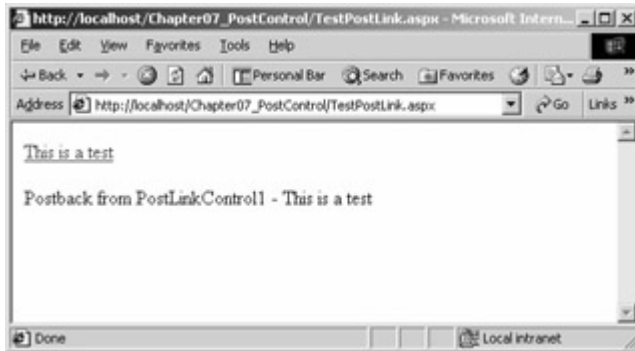
Figure 7-3 : TestPostBack.aspx after the link has been clicked and the label modified by the server code
