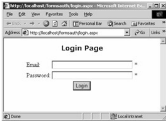
Figure 5-4 : The Login.aspx page when the Login button is clicked and the fields are not filled in
