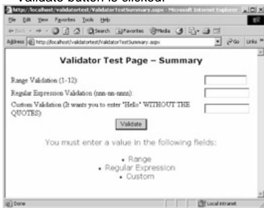
Figure 5-10 : The validation summary displayed when ValidatorTestSummary.aspx is submitted with no values entered
