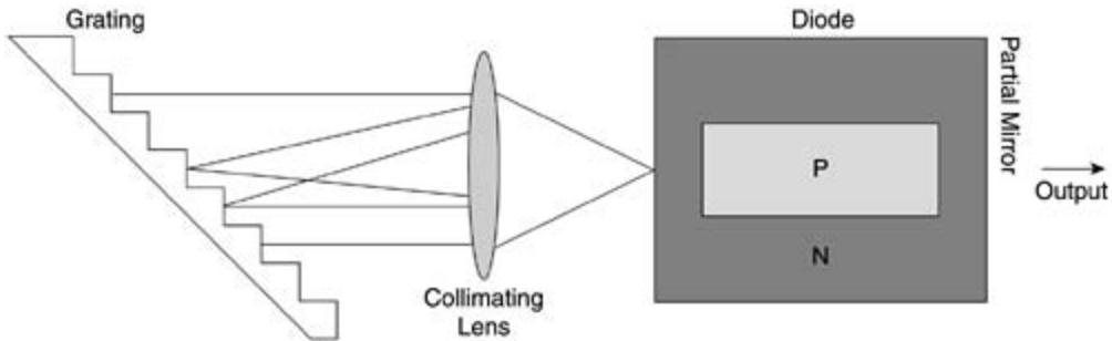
The corrugation or grating now extends to the mirrored walls, thus enhancing tunability. You can achieve wavelength tunability by varying the grating periods outside the gain medium (p-n junction). For a DBR laser, Bragg's condition given by [Equation 2-2](#) needs to be satisfied.
