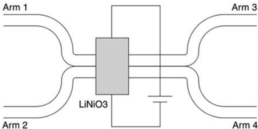
Switching times is about 1–5 ns, but loss can be almost 2–3 dB because of imperfect coupling ratios.
