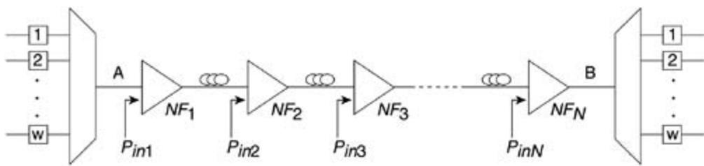
In an OSNR-based design, we must ensure that OSNR of the final stage is in compliance with system OSNR requirements and hence the BER requirements. To make the system support a particular BER, it is necessary to make the OSNR system design compliant.
