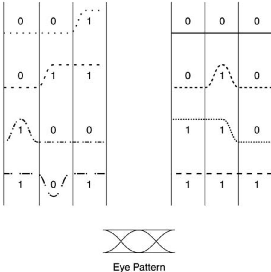
An eye diagram shows a relative performance of the signal. The horizontal and vertical openings of the eye provide valuable information about the ability of the receiver to detect a 1 bit and a 0 bit correctly. [Figure 9-26](#) shows the characteristics of the eye diagram. The vertical *eye opening*
