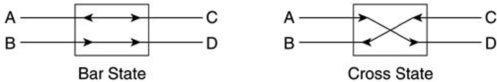
The advantage that micro-mechanical switches offer is that they are fairly robust and inexpensive. Presently, many vendors use such switches in network elements because of their low cost and comparative performance. These switches have negligible wavelength dependent loss and work quite the same for different wavelengths.
