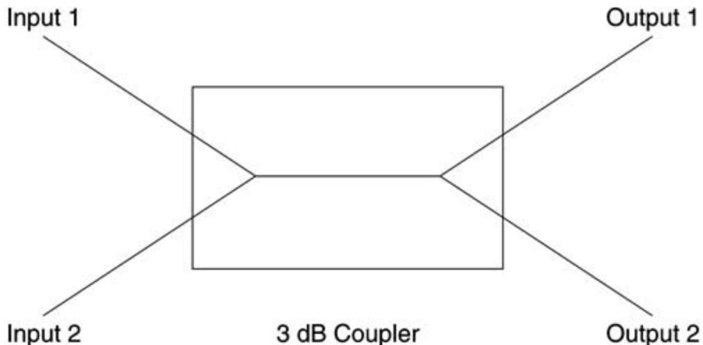
Couplers find applications for monitoring WDM ports as well as for passively adding channels into a fiber. They are also used in passive optical networks (PONs) as a method to provide shared medium access (Ethernet PON, or EPON).
