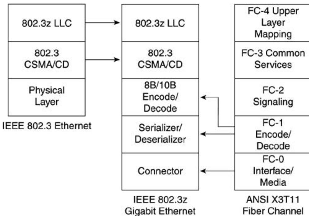
The serializer/deserializer is responsible for encoding schemes and communication to the upper layers. The encoding scheme used in 802.3z is 8B/10B, which is similar to fiber channel encoding.
