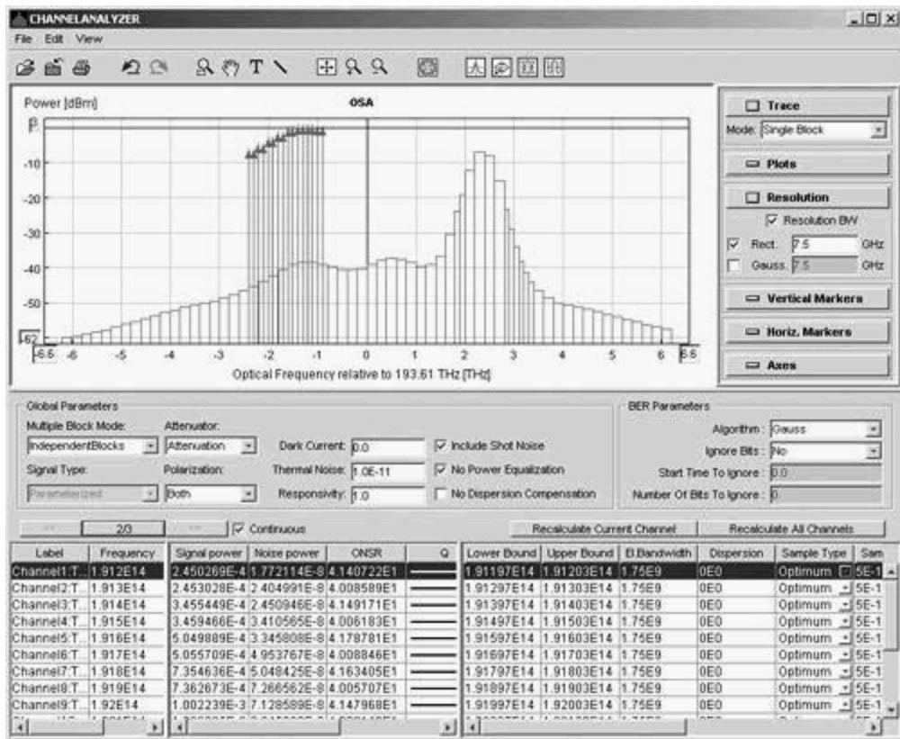
Figure 10-7. Iteration of Input Powers to Achieve Equal SNRs. At Iteration 2, the SNRs have crossed over because the Spectral gain of an EDFA is a function of input power.
