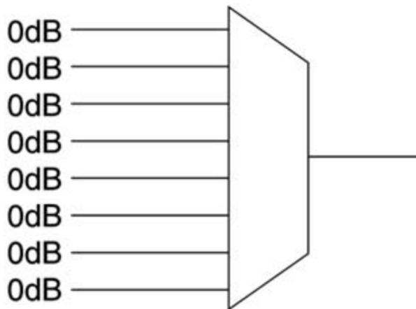
$$P_{\text{composite}} = P_{\text{channel}} + 10\log N - \text{Insertion loss} \quad (\text{where } N \text{ is the number of channels})$$
