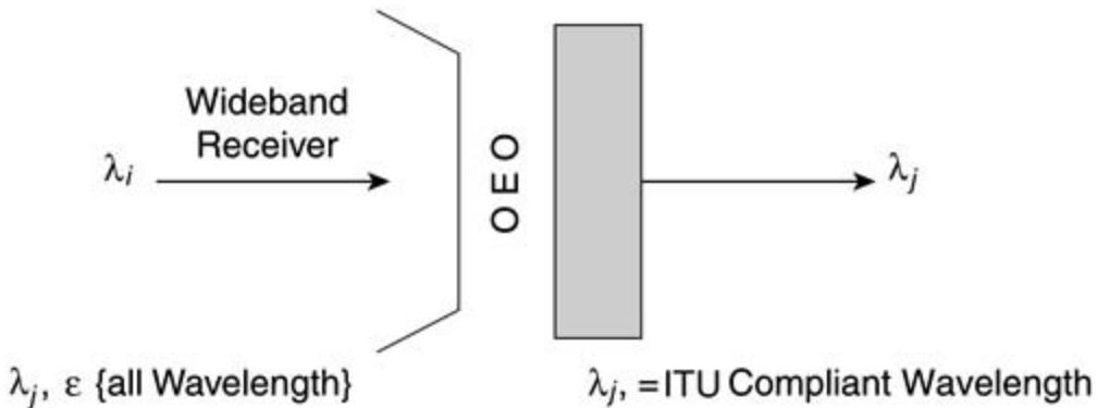
Because of the O-E-O symmetry, transponders usually perform 3R regenerations, but 2R generations are also possible. (3R transponders are not bit-rate transparent.) For example, an OC-48 transponder cannot be used for an ESCON or a FICON (SAN interfaces). Configurable 3R transponders are available in the market today; an interface can be configured to OC-48/OC-12/OC-3/GigE.
