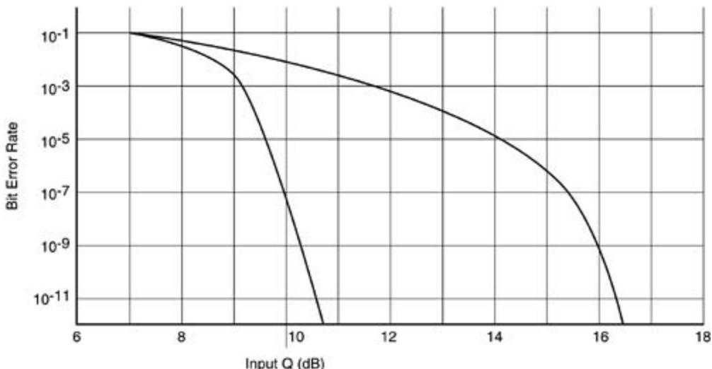
[Figure 4-4](#) shows the penalty of the Q-factor due to nonlinear effects by increase in input power.
