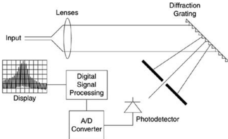
The filtered signal falls on a photo detector, which then converts the optical signal into an electrical signal. The signal is then fed into an Analog to Digital (A/D) converter. Finally, the signal is processed by a digital signal processor and displayed on the scope. A simplified block diagram of a diffraction based spectrum analyzer is shown in [Figure 9-7](#). A real spectrum analyzer is more complex with circuits, analyzing and controlling functions.
