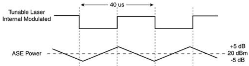
The OSA is then gated to produce measurement in both signal-off and signal-on conditions. The signal-off spectrum allows the direct determination of ASE. [Figure 9-21](#) shows the signal-off and signal-on conditions. This is an accurate method for measuring the NF of EDFA amplifiers. This technique will not work with SOA and Raman amplifiers.
