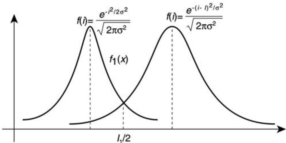
The deviation threshold can be further optimized to reduce BER. This is obtained when condition as in [Equation 2-35](#)<sup>2</sup> is met.
