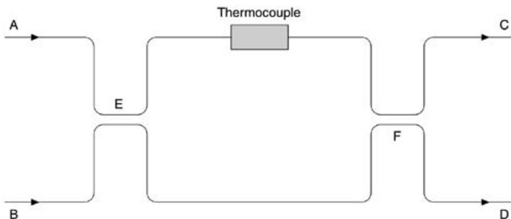
Such devices switch signals as follows. Consider [Figure 2-36](#). Signals A and B are made to interfere at point E such that B interferes destructively; therefore, at point C, only A will appear. Similarly, A can be made to switch to port D by destructively interfering at point F. Such switches are slow and have high cross-talk due to an imperfect coupling effect.
