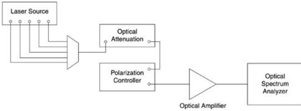
The laser sources are used as input channel to the optical amplifier under test. The laser sources can be DFB lasers or tunable lasers (DBR). The variable attenuators vary the power for different input power selections, and the polarization controllers randomize the state of the polarization. The OSA displays the result in a graphical form.
