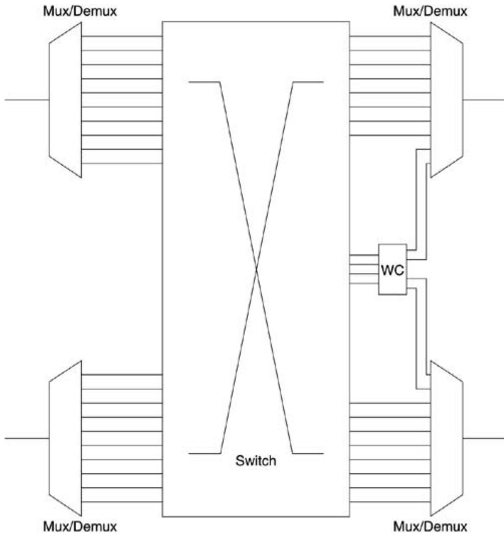
Overall, wavelength conversion for metro networks was not a feasible idea. To a great extent, this diminished the advantages of a cross-connect architecture over the conventional OADM add/drop architecture.
