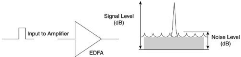
The noise is random in nature, and it is accumulated at each amplification stage. Refer to [Figure 4-2](#).
