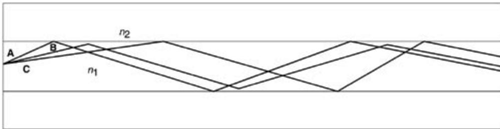
Rays A, B, and C can be considered as three modes of propagation that are each defined by a propagation constant  $\beta$ . Further, each mode has a wave number.
