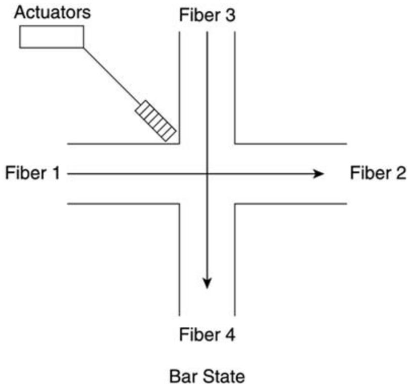
Four fibers (1, 2, 3, and 4) are coupled together to form a  $2 \times 2$  cross-connect. A double-sided mirror that is perpendicular to the plane of the page is present and held in position by two actuators. In the bar state, light from fiber 1 is coupled to fiber 2, and light from fiber 3 is coupled to fiber 4.
