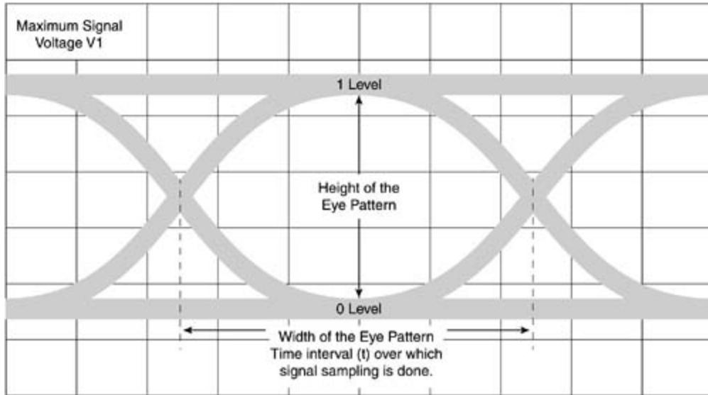
For a good transmission system, the eye opening should be as wide and open as possible. The eye diagram also displays information such as maximum signal voltage, rise and decay time of pulse, and so on.
