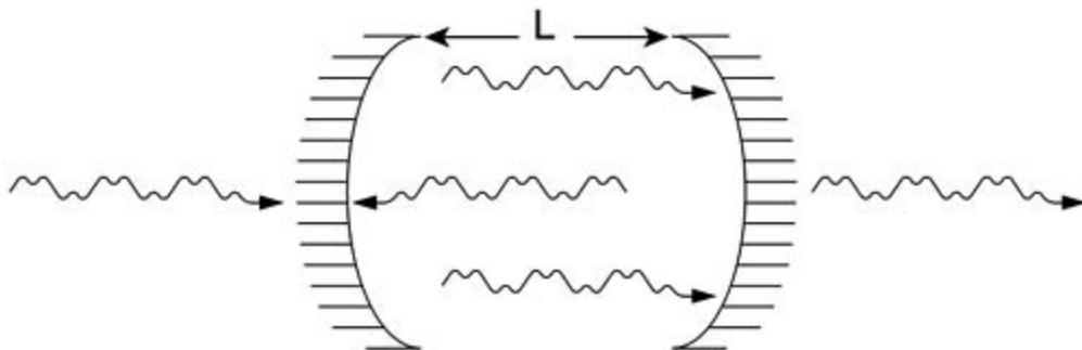
The transmission characteristics or the transitivity of an FP cavity is best for  $\lambda = \lambda_{\text{resonance}}$ , which is generally shown as in [Equation 2-43](#).
