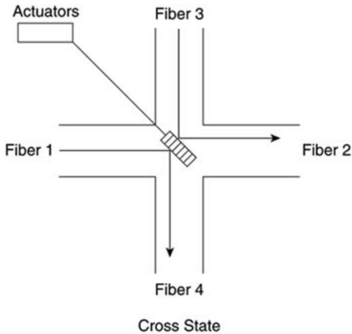
Typical switching times are in millisecond range. The insertion loss of the switch is about 1 dB per port. MEMS switches can be scaled to provide an  $N \times N$  cross-connect. The one shown in [Figures 2-32](#) and [2-33](#) is a 2D MEMS (2-dimensional MEMS). In contrast, [Figure 2-34](#) shows a 3D MEMS switch (3-dimensional). The incident light in 3D MEMS is switched in 3D space using collimated lens to provide efficient 3D switching; it is comparable to free space optics.
