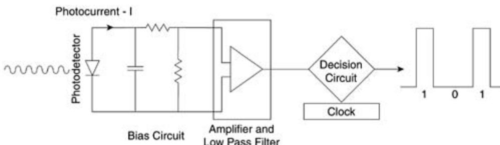
An optical receiver consists of a photodetector followed by a preamplifier. The function of a preamplifier is to amplify the photocurrent for further processing. The next stage consists of a high-gain amplifier and a low-pass filter. An amplifier gain control circuit automatically limits the amplified output to a fixed level, regardless of the optical power incident on the photodetector.
