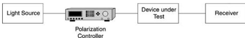
Polarization dependent loss can be defined as the difference in the maximum and minimum variation in loss (transmission/embedded) of an optical device over all states of polarization (SOP) and is expressed in dB.
