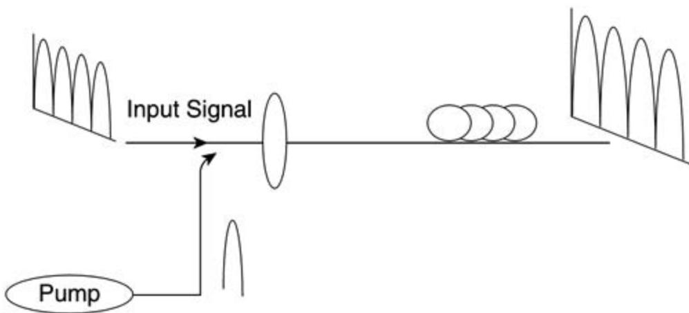
In other words, energy is transferred from a pump to a Stokes wave, and the number of photons in a pump wave and a Stokes wave remains constant. A figure of merit in the functioning of Raman amplifiers is the *Raman threshold*, defined as the amount of pump power needed to make the pump equal to the power of a Stokes' wave<sup>2</sup>. Raman threshold is also subject to a
