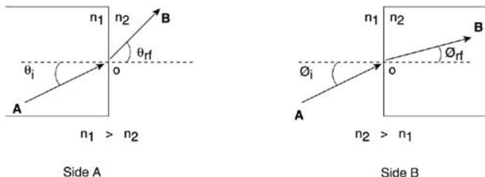
If the angle of incidence of a ray of light, in a denser medium is continuously increased, the corresponding refracted ray (in the rarer medium) is bent away from the normal; this "away bending" can be mathematically explained by Snell's law (see [Equation 1-2](#)). As we increase the
