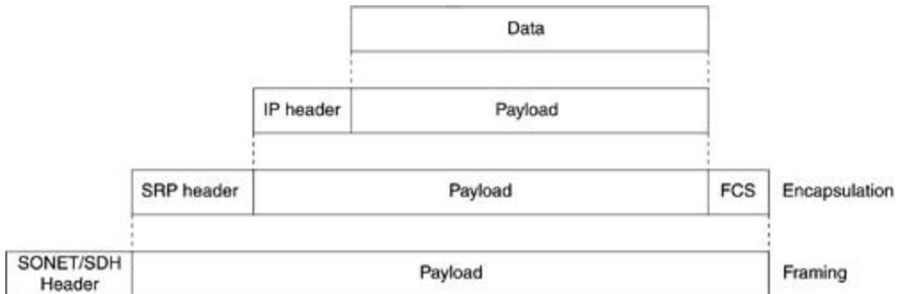
The transmission rates currently defined are OC-12/STM-4, OC-48/STM-16, and OC-192/STM-64 for the SRP/DPT interfaces. Most of the implementation currently is based on OC-12/STM-4 or OC-48/STM-16, but OC-192/STM-64 is gaining popularity. The OC-192/STM-64 interface is deployed on the GSR 12400 series routers.
