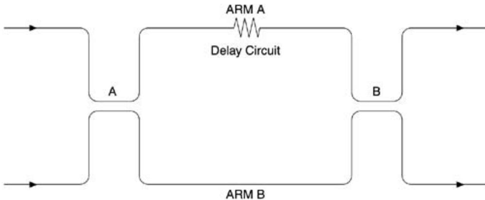
The two propagating signals can be made to obtain different phase shifts by varying the lengths of the two arms. The signals, upon interfering with each other at coupler B, might have constructive or destructive interference. The phase shift induced is a frequency (hence wavelength)-dependent quantity  $\phi(f)$ , shown in [Equation 2-46](#).
