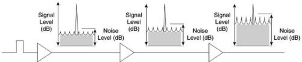
Amplifier noise is a severe problem in system design. A figure of merit here is the optical signal-to-noise ratio (OSNR) requirement of the system. The OSNR specifies the ratio of the net signal power to the net noise power. It is a ratio of two powers; therefore, if a signal and noise are both amplified, system OSNR still tells the quality of the signal by calculating this ratio. System design based on OSNR is an important fundamental design tool.
