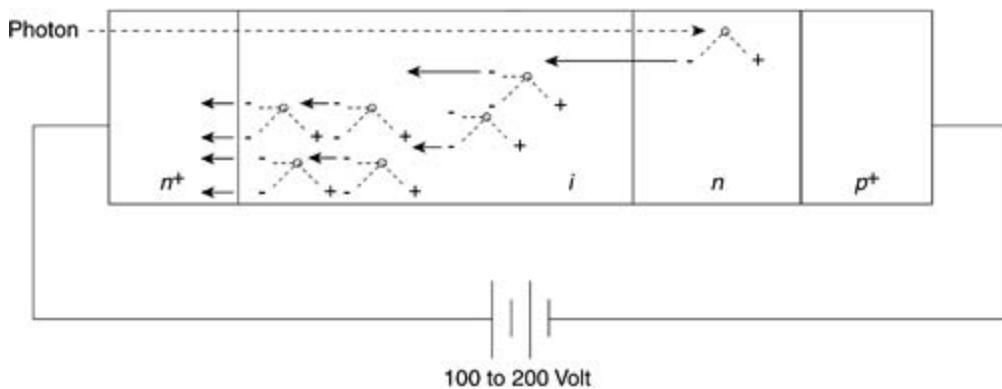
In practice, the avalanche effect is a statistical phenomenon. In other words, electron hole pairs generated by the primary electrons are randomly distributed. The statistical value is termed as *multiplicative factor*, or multiplicative gain ( $M_f$ ), and is shown in [Equation 2-6](#).
