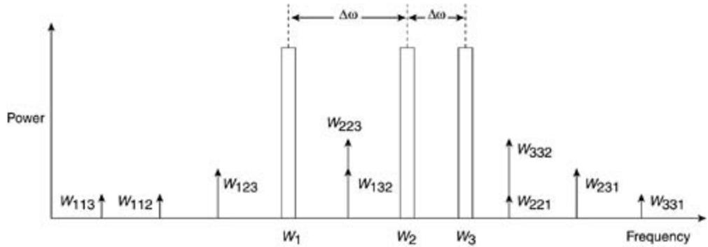
The solution for minimizing FWM is to use unequal channel spacing in such a way that the generated wavelength does not interfere with the signal channel(s). Use of NZDSF minimizes the effect of FWM.
