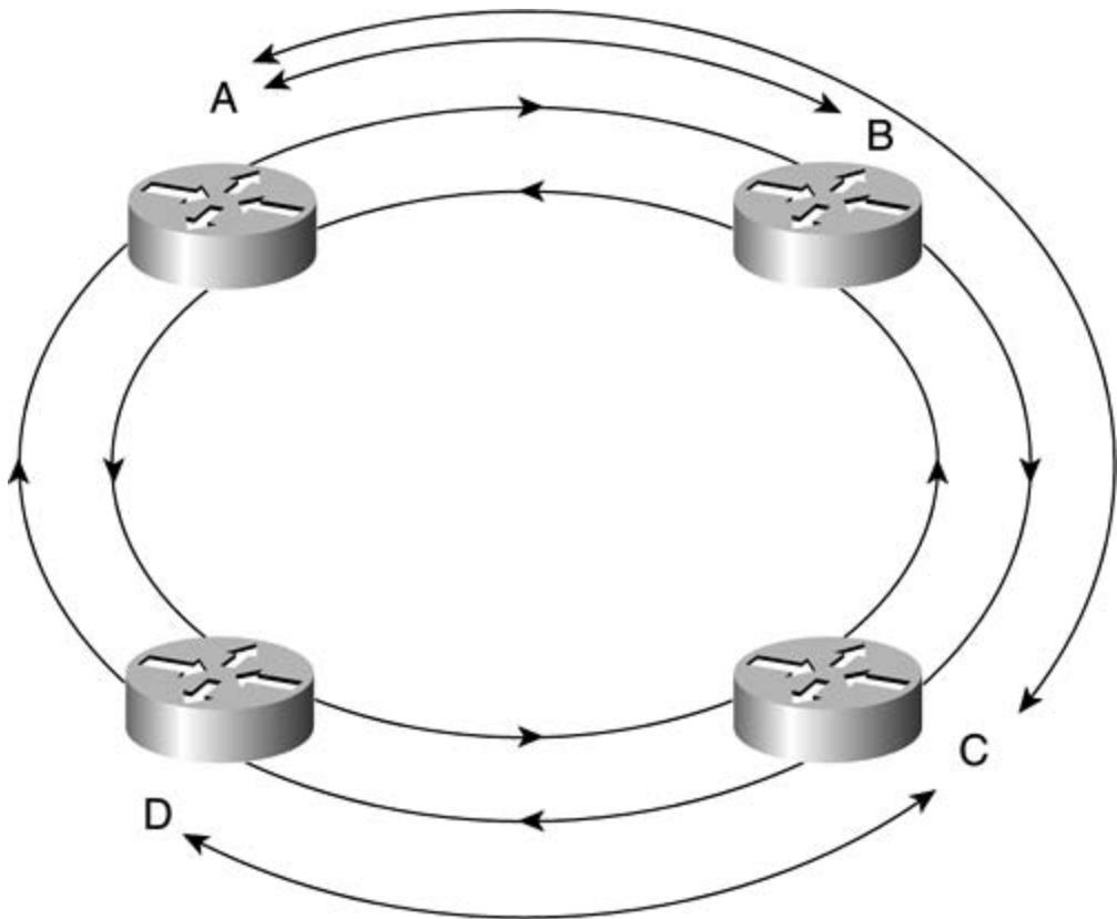
SRP is a media-independent media access control (MAC) layer protocol. The initial implementation utilizes SONET/SDH framing so that interworking with current SONET/SDH infrastructure is possible. A typical SRP frame is shown in [Figure 7-23](#). Each SRP interface has a unique 48-bit IEEE MAC address (Ethernet-like MAC address). A multicast bit is also defined to support multicasting. In multicasting mode SRP, the source strips the multicast packet (not destination stripping).
