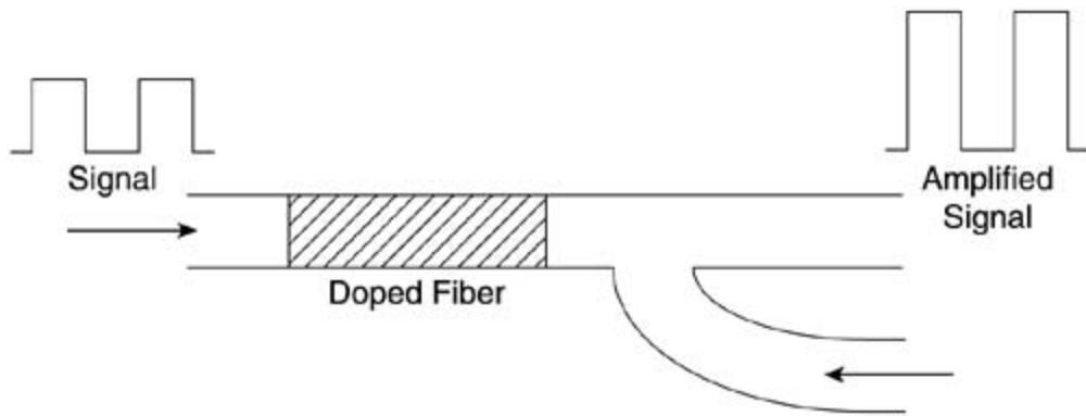
A third example is when two pumps are applied<sup>7</sup> and are in forward and reverse direction at the same time; this method is known as *bidirectional pumping*. Power conversion efficiency (gain per input pump power) is exhausted in a backward (reverse) pumping direction. In bidirectional pumping, the gain profile throughout the doped region is almost linear, which is an advantage. See [Figure 3-5](#) for a view of bidirectional pumping.
