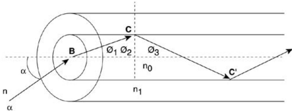
From Snell's law, it is possible to calculate the maximum angle that the incident ray can make with the axis OO' so that it remains within the periphery of the core (gets contained in the core).
