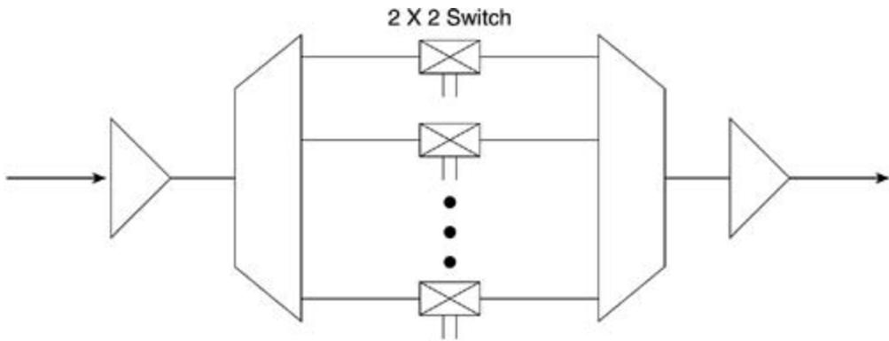
As of today, most networks are circuit switched, so they work well with mechanical switches. Mechanical switches have a typical switching time (from one state to another) of 10–15 milliseconds. This is enough to ensure 50-millisecond restorations, as in SONET-like networks after fiber cuts. Metro networks can also be built without full demultiplex sections.
