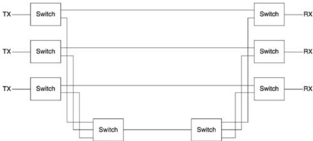
Naturally, the 1+1 protection format is a much easier way of guaranteeing fast protection (restoration time is minimal), but the cost involved is often more as more bandwidth (resources) is needed to facilitate it. 1:1 protection, in contrast, is not that fast in terms of restoration time (time needed to restore a failed link or lightpath), but the cost involved is often quite lower even though the signaling procedure is often cumbersome because of the fact that
