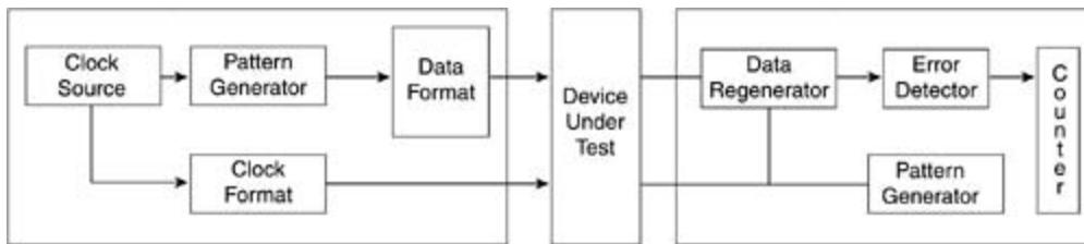
The error-detection circuit verifies that each bit sent through the device under test has been correctly received. The error detector and the signal pattern are synchronized and compared bit for bit. Whenever there is a discrepancy, an error is counted. Therefore, BER is determined from the number of bits found in error and the total number of bits verified.
