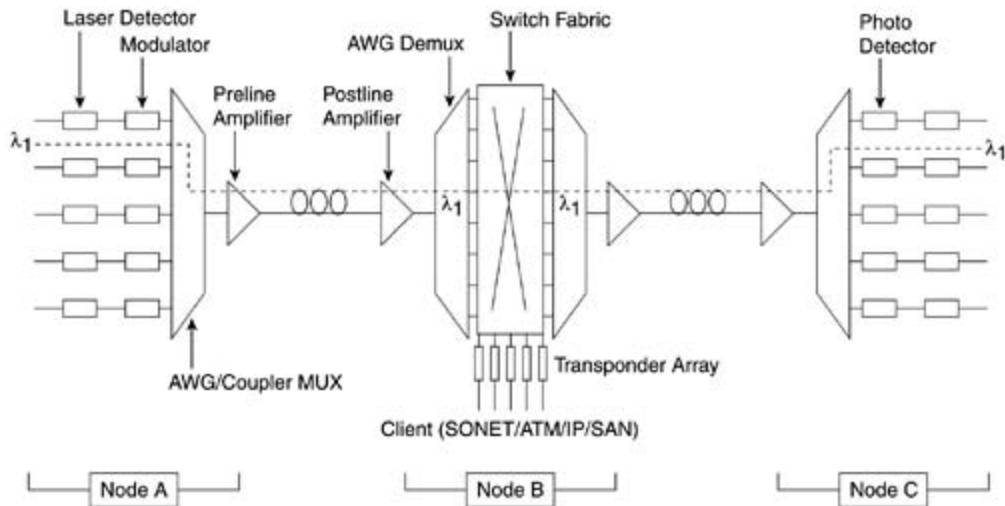
At node A, an array of electrical data devices injects data into different wavelengths. These devices could be SONET platforms, ATM switches, or even routers. (IP over DWDM is explained in [Chapter 7](#).) The electronic data is modulated onto an optical channel at a specified wavelength.
