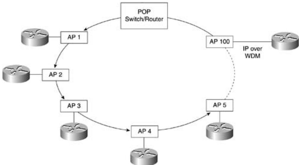
The network is designed to scale to 100 access points and ring circumference of around 100 km with a bit rate of 2.5 Gbps. A subcarrier multiplexing technique is used to carry control information, which includes access point addressing and wavelengths. Multihopping is supported with this architecture, which also helps the network scale efficiently. Access points can use any wavelength, and wavelength bandwidth is shared statistically among various access points.
