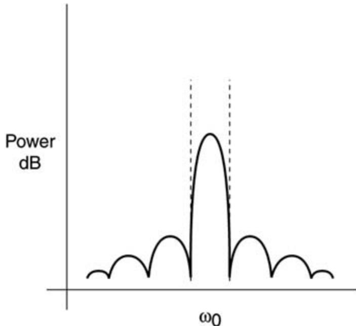
The typical line width for WDM systems is in the range of a few megahertz. Laser line width is a major issue in WDM systems; the greater the line width, the greater the cross-talk with adjacent channels and the greater the nonlinear effects that are associated.
