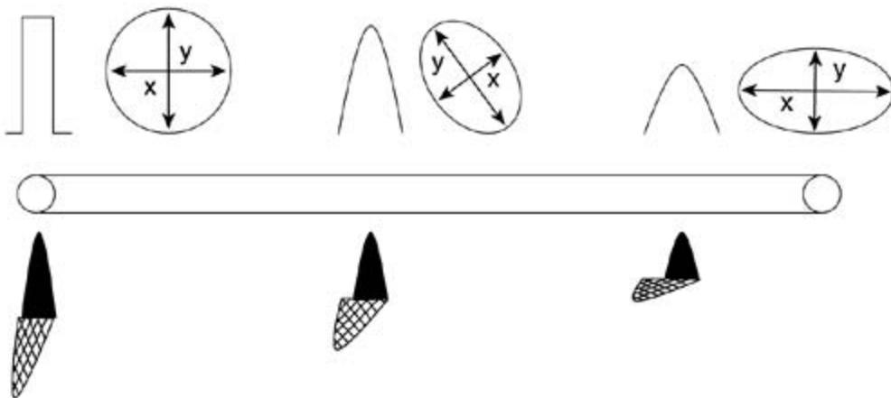
[Figure 1-11](#) shows PMD resulting from the effects of a fiber acquiring birefringence and the energy transfer between the two polarized modes, leading to pulse spread.
