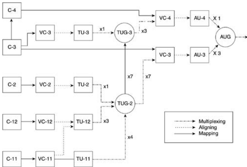
[Figure 7-17](#) shows how a C-4 container is mapped and how an STM-1 signal is formed.
