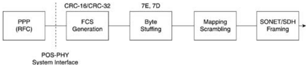
In addition to high bandwidth, POS offers reliable and secure data transmission. The data is scrambled using an ATM-like scrambler, self-synchronized payload scrambler, which is defined by RFC 2615. When POS is connected to the SONET/SDH network, the timing is derived from the SONET/SDH network. When POS is connected through dark fiber or DWDM, timing is derived from the internal clock. (Links are independently timed by 20-ppm internal clock built into the POS interface.)
