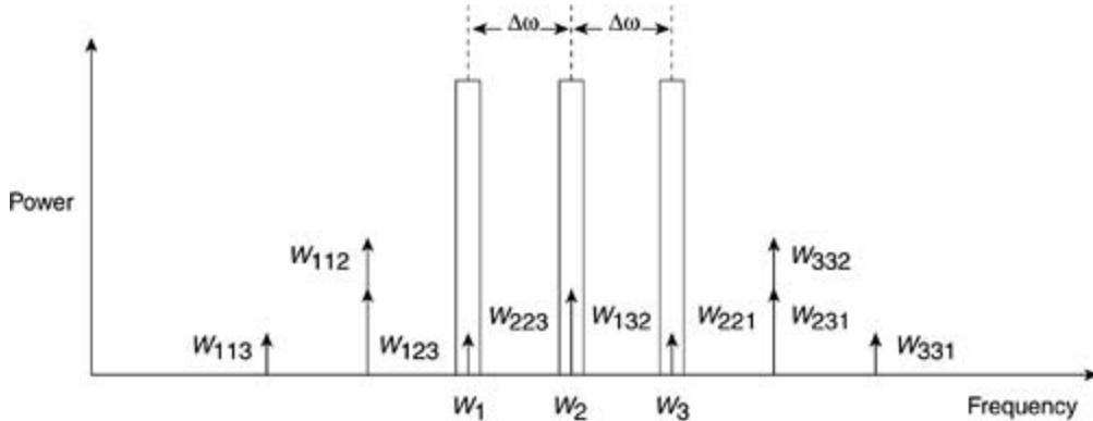
Figure 4-13. Three Unequal Spaced Channels Generating Nine FWM Signals; None of the Generated Signals Falls on Top of the Original
