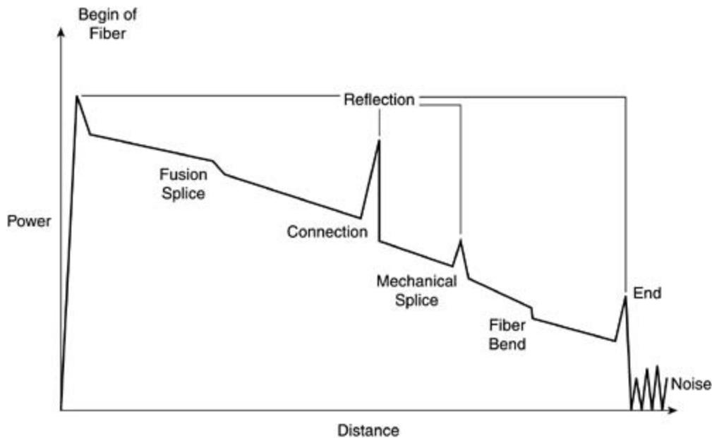
From the trace in [Figure 9-11](#), we can see a small level of attenuation and strong reflection at
