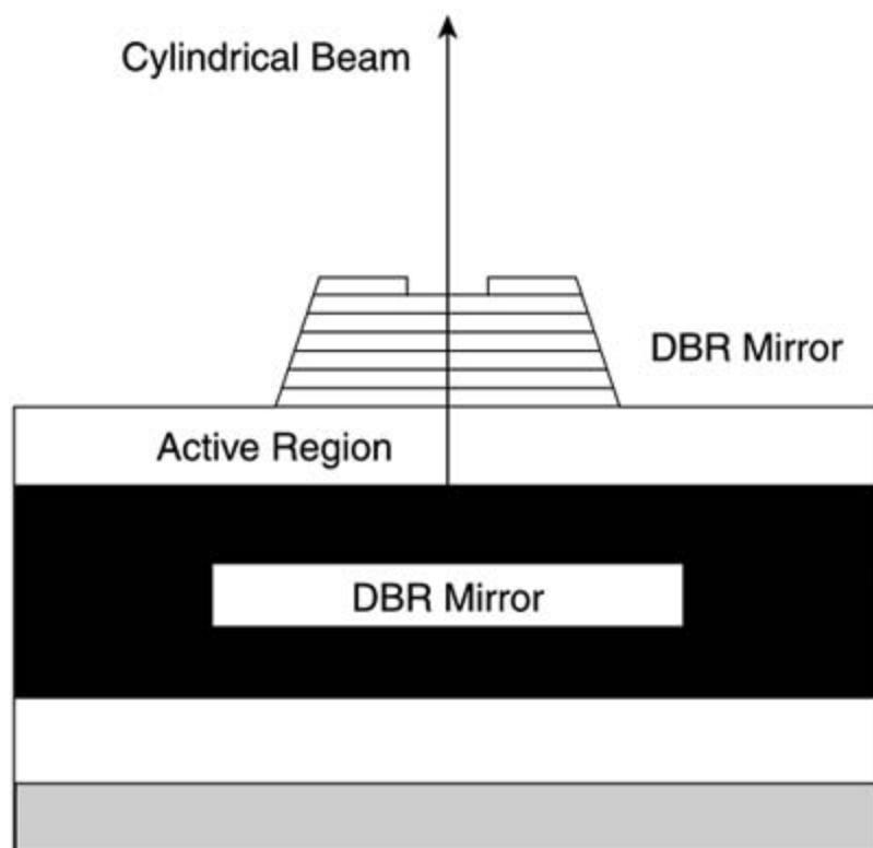
A VCSEL is composed of many specialized layers, analogous to edge-emitting lasers. The main parts of a VCSEL are the active region and the mirrors. A sandwich of active regions (between the mirrors) is created by stacking the subcomponents vertically on top of each other. For fiber-optic communication, VCSEL uses Indium Gallium Arsenide Phosphide (InGaAsP) for wavelengths of 850 and 1310 nm.
