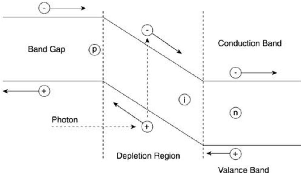
To generate the photocurrent, we must ensure that the energy of the incident photon is equal to or greater than the bandgap energy.
