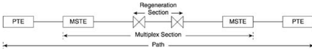
The section layer (SONET/Regeneration Section, or SDH) is responsible for transport of STS-N /STM-N frames across the network media. This layer's functions include framing, scrambling, maintenance, and error monitoring. The photonic layer is where the conversion of the signals happens before the signal is transported through the fiber. This layer determines the launch power, shape, and frequency of the optical pulse.
