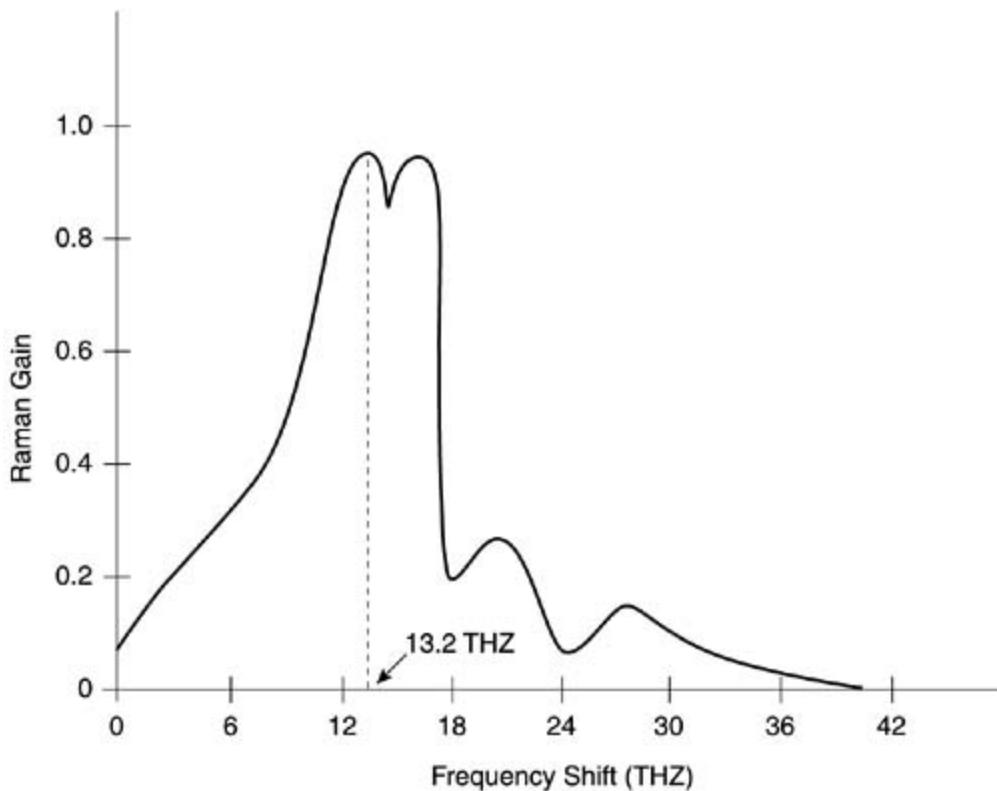
Figure 3-7. Raman Amplification
