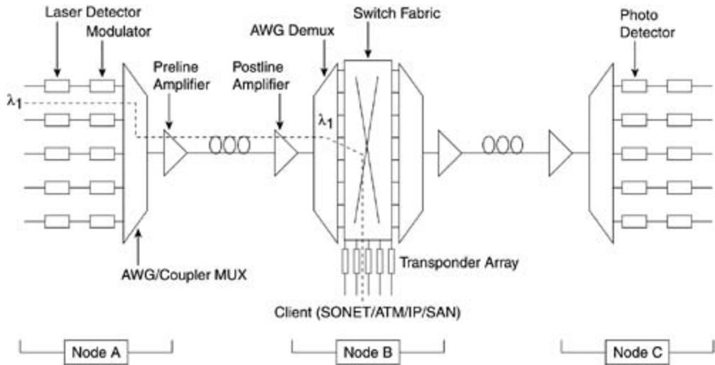
In summary, the switch fabric does the task of adding, dropping, or switching optical channels or even just passing them through (pass through functionality). The channels are then fed to a multiplexer and recombined into a composite WDM signal. This signal is amplified by the pre-line fiber amplifier.
