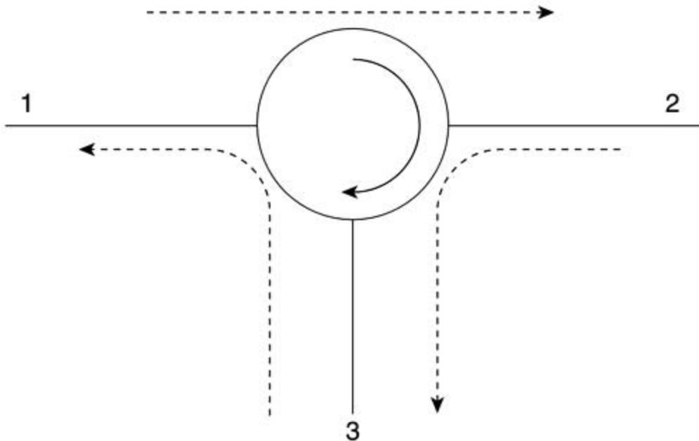
A circulator is a multiport device that allows signals to propagate in certain directions based on the port that the signal came from (incident port). The operation is based on an isolator (analogous to an optical valve), which allows unidirectional propagation only. In [Figure 2-21](#), the signal from port 1 moves freely to port 2; while the signal from port 2 cannot go to port 1, but it can go to port 3. Likewise, the signal from port 3 can go to port 1 but not to port 2.
