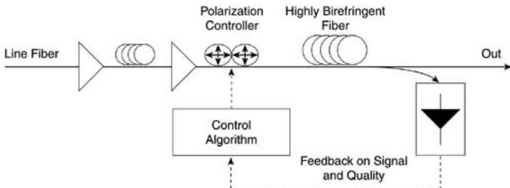
The control algorithm is in a tracking mode and operates in blind mode-PMD conditions are not dynamically controlled; Control algorithm has to keep track of local optimum feedback signals.
