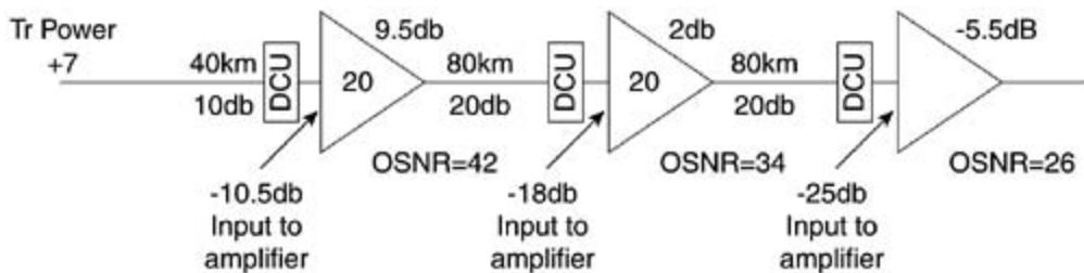
Step 1. The total distance is 200 km; therefore, total loss is  $200 * .25 = 50 \text{ dB}$ . You need amplifiers to reach that distances.
