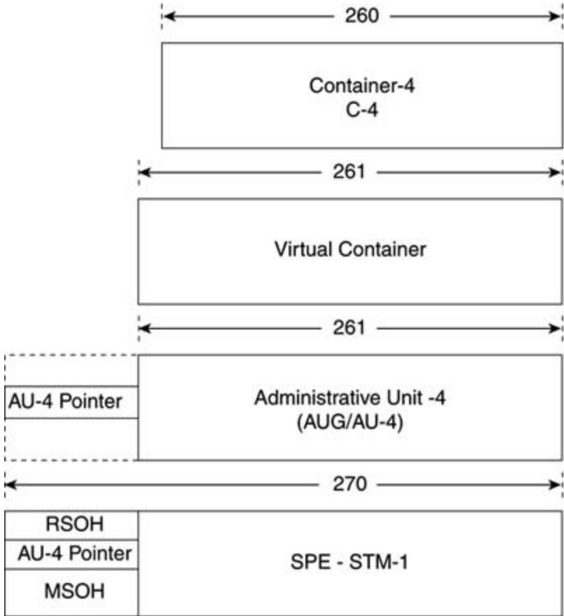
The C-4 container occupies 9 rows and 260 columns. As explained before, VC-4 is obtained by adding a row of path over head (POH) to C-4 signal. To VC-4 signal, a 9 byte of AU-4 pointer is added to get the AU-4 signal. Transport overhead (RSOH and MSOH) is added to AU-4 to get the STM-1 signal.
