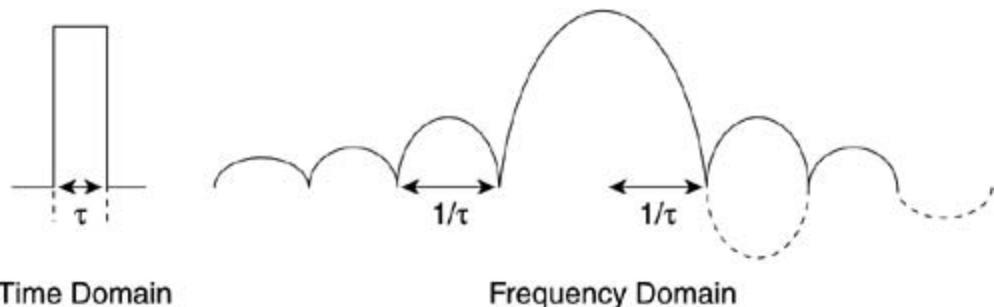
For the same data rate Return to Zero (RZ) has half the pulse width of that of NRZ (see [Figure 8-5](#)).
