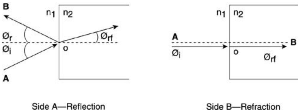
In [Figure 1-1](#), section A, AO represents a ray incident on a denser medium from a rarer medium. A denser medium is one of high material density and also high refractive index; in contrast, a rarer medium is one with lower index and lower density. OB represents the reflected ray. In [Figure 1-1](#), section B, OB represents the ray that passes through when the angle of incidence is 0 degrees to the normal.
