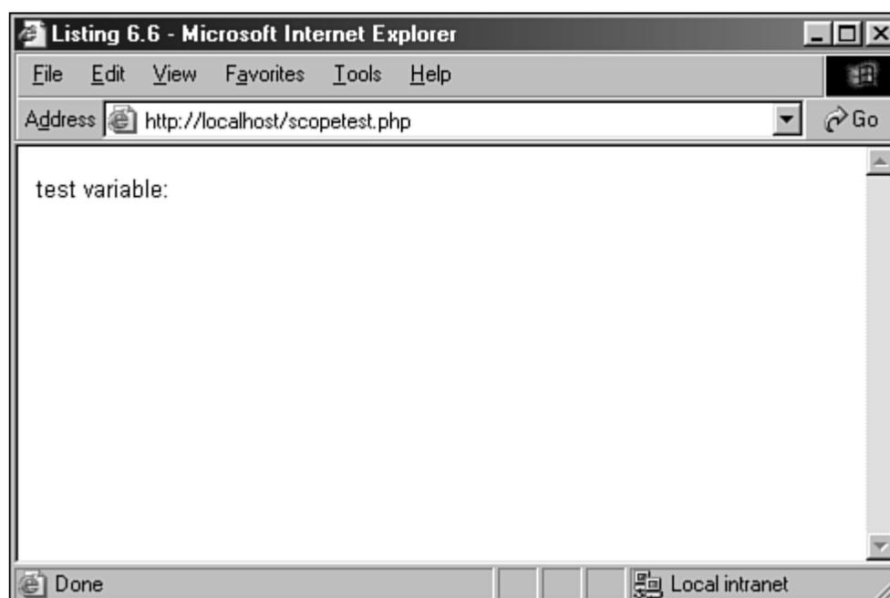
The value of the variable `$testvariable` is not printed. This is because no such variable exists outside the `test()` function. Note that the attempt in line 10 to access a nonexistent variable does not cause an error.
