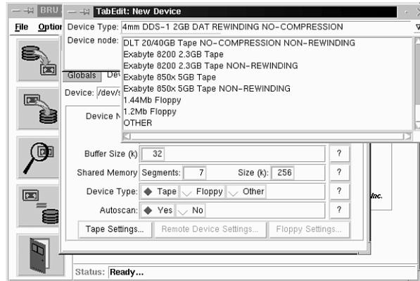
There are 37 different devices listed, including floppy drives. If you don't see a device you have in the list, select the OTHER device option to create your own. For example, if you have an older, floppy-based tape drive that uses the QIC-80 format, select OTHER and specify the tape device (most likely `/dev/rft0`, the rewinding tape device).
