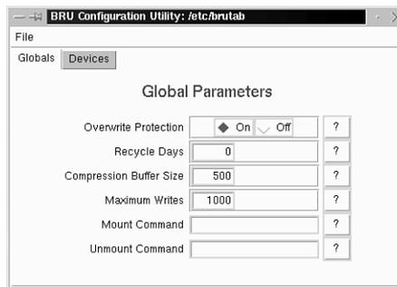
Click the Devices button in this window, and then click the New button. A New Device window, as shown in Figure 23.3, with a scrolling list of different devices appears.
