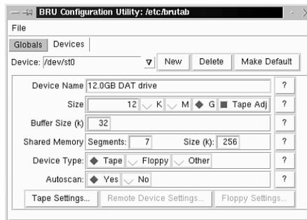
Click the New button to select a new device from BRU's built-in list, as shown in Figure 23.4.
