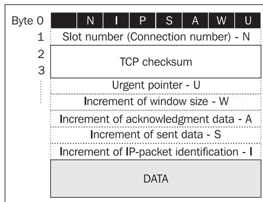
Figure 4.5: Compressed header
