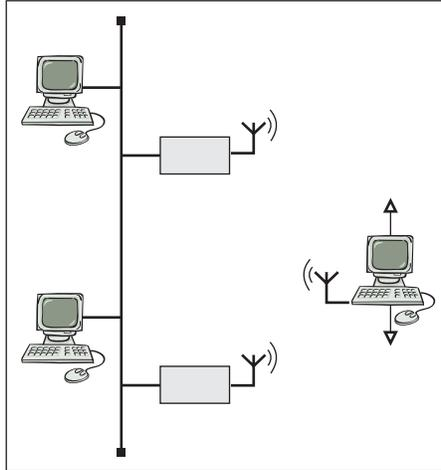
Figure 4.44: Roaming WLAN
