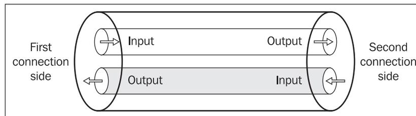
Figure 9.1: TCP creates a fully two-way link between the ends of the connection
