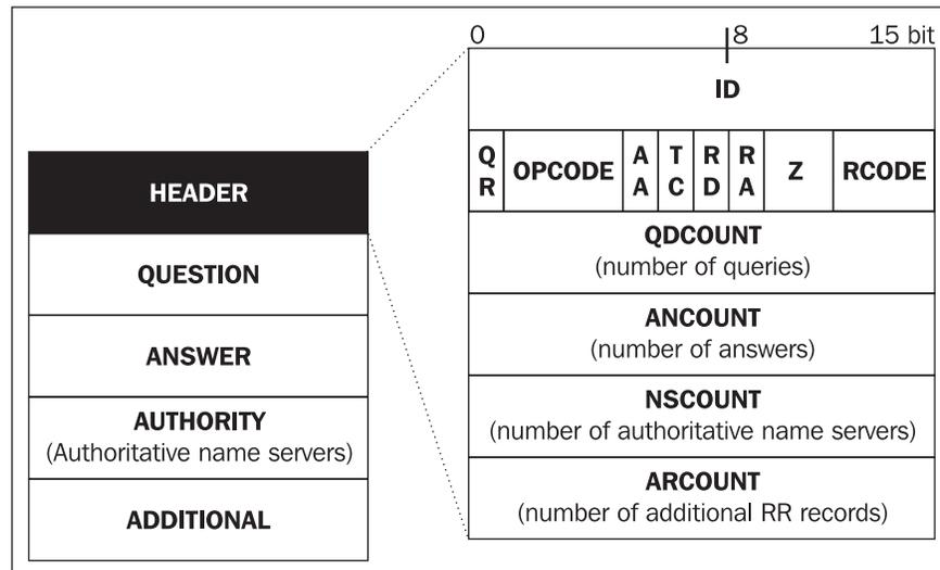
Figure 11.4: DNS Query packet format
