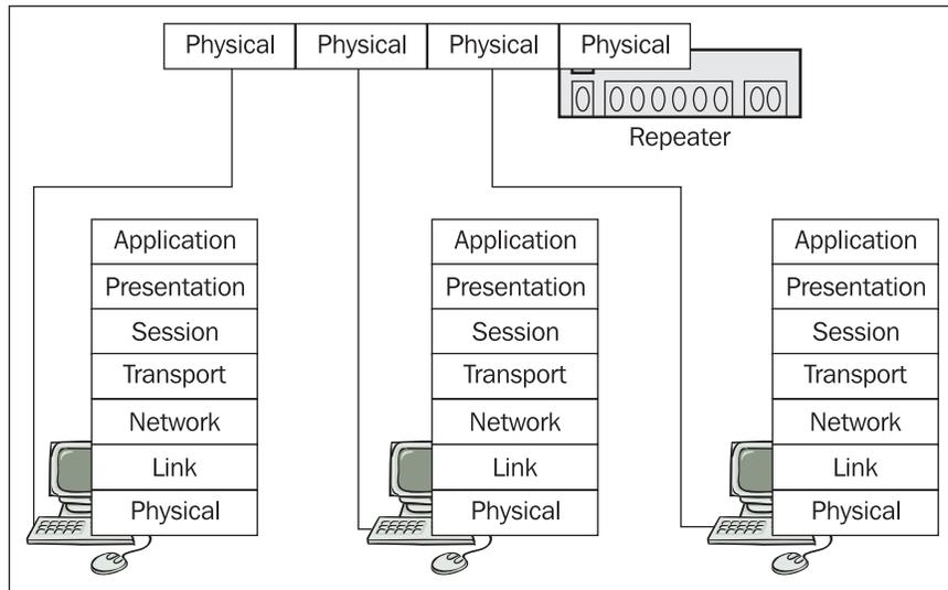
Figure 4.35: Repeater for twisted-pair
