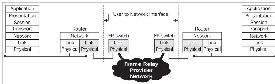
Figure 4.24: Interconnection through the Frame Relay provider
