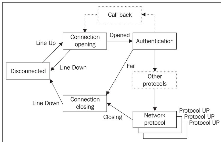
Figure 4.14: Individual link phases in PPP
