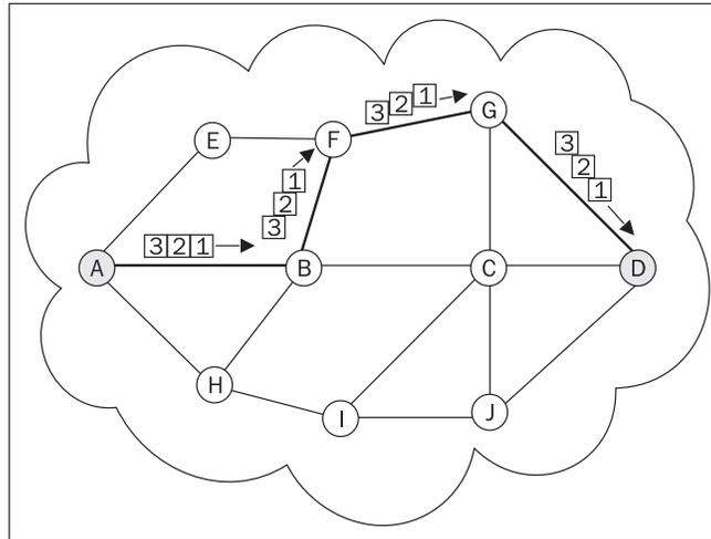
Figure 1.16: Virtual circuit
