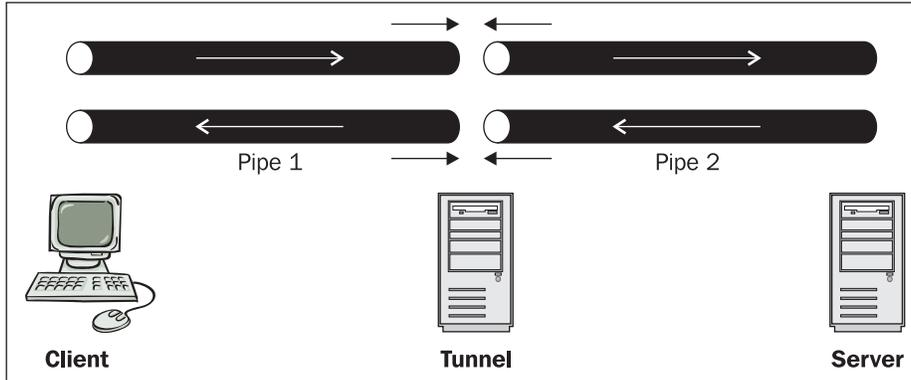
Figure 14.8: A tunnel welds both connections together
