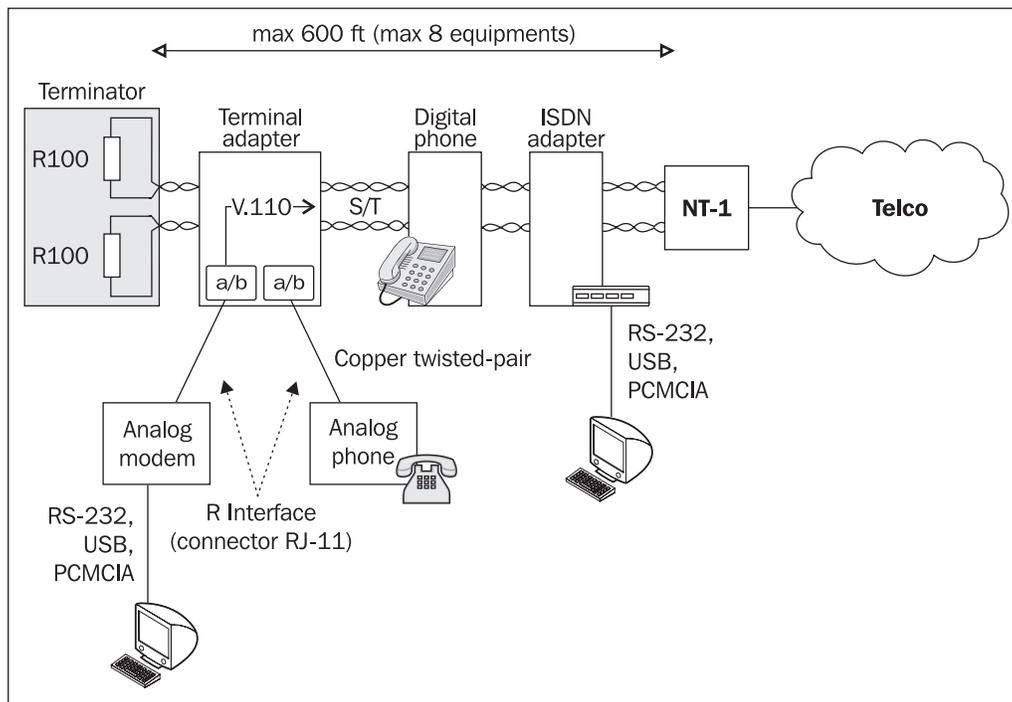
Figure 3.16: Connecting appliances to the S/T interface
