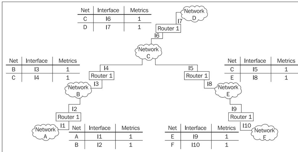
Figure 7.6: The first step of filling routing tables
