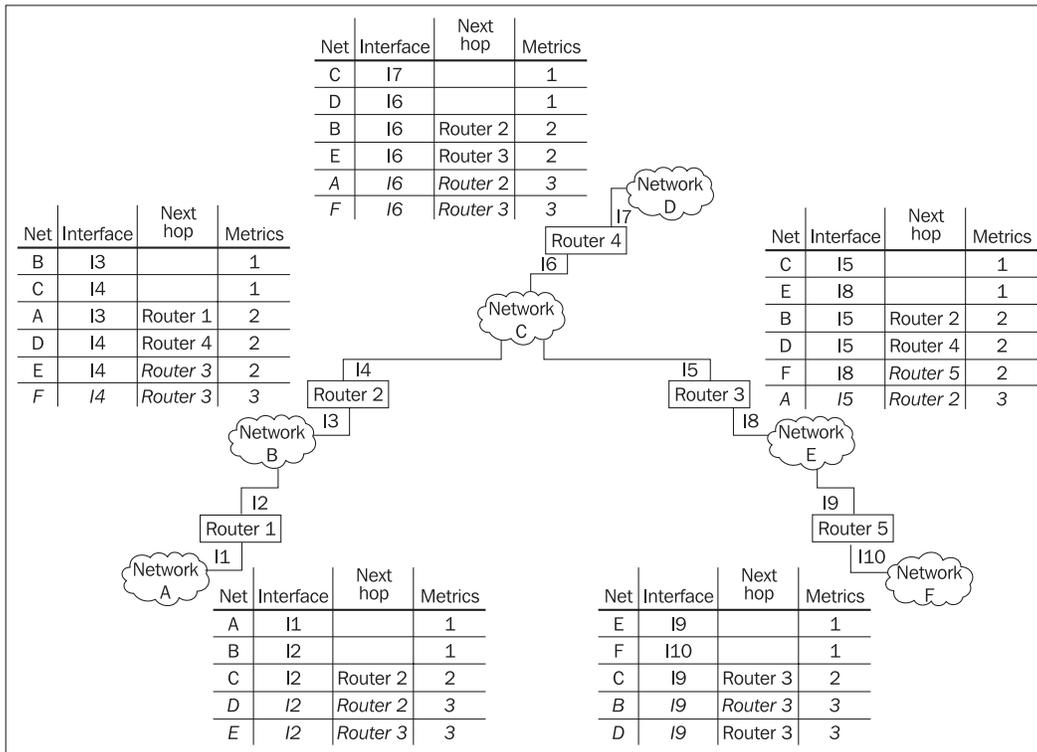
Figure 7.8: The third step of filling routing tables
