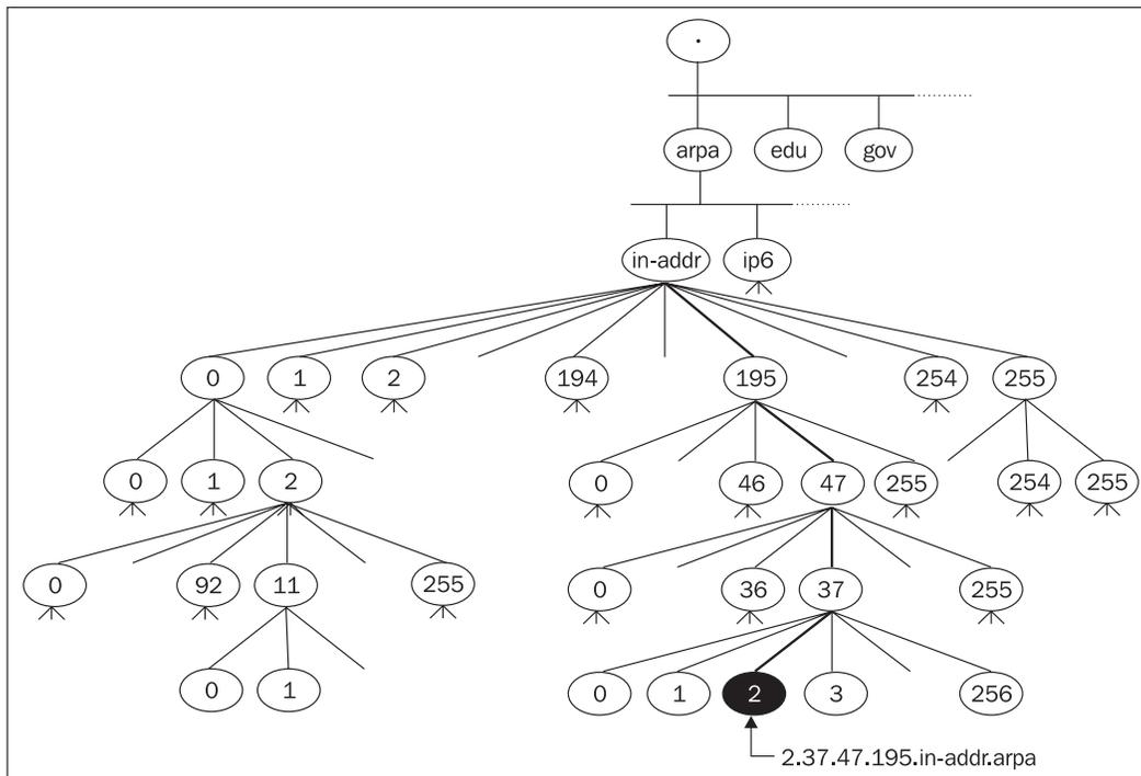
Figure 11.2: Reverse domain to IP address 195.47.37.2
