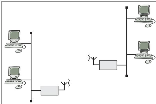
Figure 4.45: Backbone point-to-point connection
