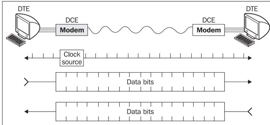
Figure 3.2: Synchronous transport
