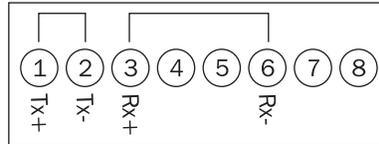
Figure 3.32: Connecting the outlets for 10BASE-T or 10BASE-TX
