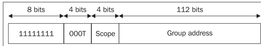
Figure 8.19: Multicast address
