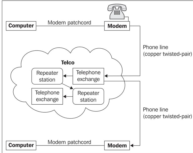
Figure 3.9: Baseband modems using a direct metallic connection
