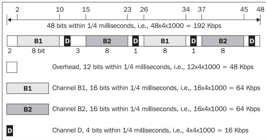
Fig. 3.17: Basic Rate divided into individual slots
