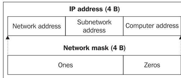
Figure 6.3: IP address and its network mask
