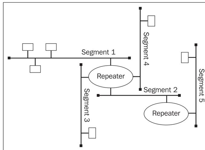
Figure 4.33: LAN consisting of individual segments
