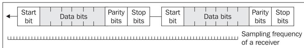
Figure 3.1: Asynchronous arrhythmic character transport
