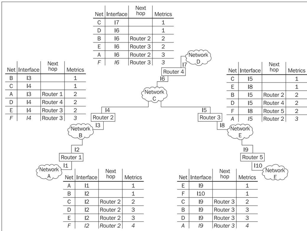
Figure 7.9: The fourth step of filling routing tables
