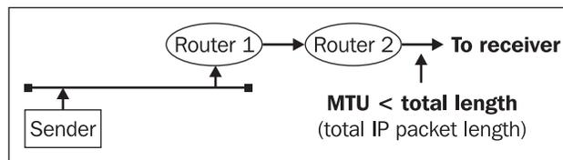
Figure 5.14: MTU between the router and the recipient
