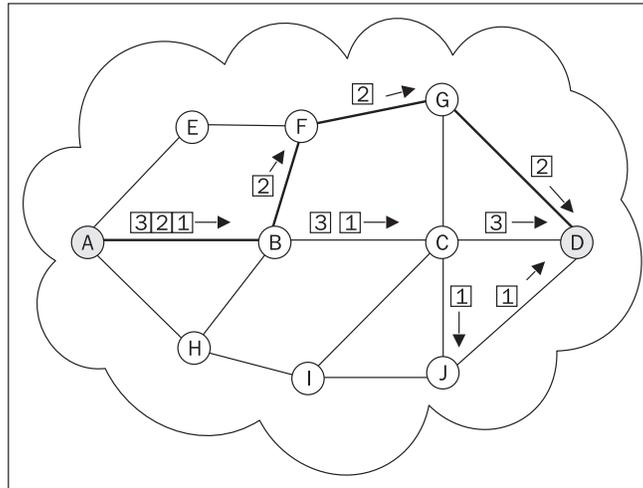
Figure 1.17: IP does not use virtual circuits.
