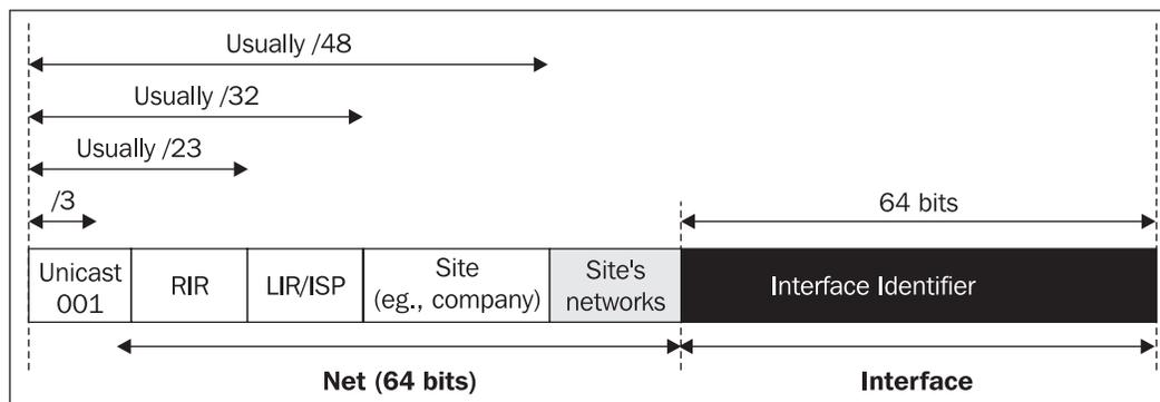
Figure 8.20: Unicast IP version 6 address assignment
