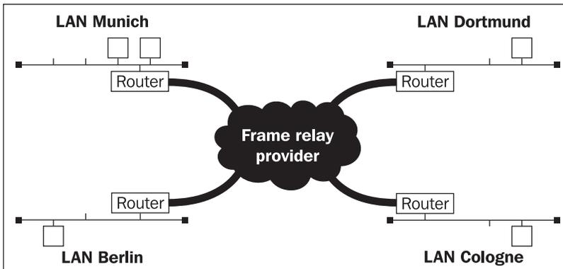
Figure 4.22: WAN based on Frame Relay
