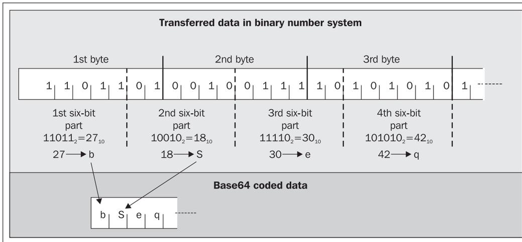
Figure 15.5: Base64 encoding
