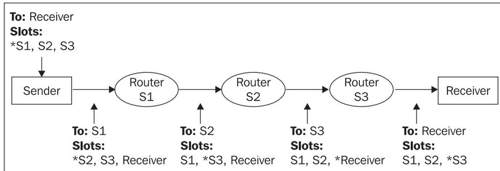
Figure 5.22: Source routing
