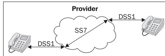
Figure 3.19: DSS1 and SS7 signalization
