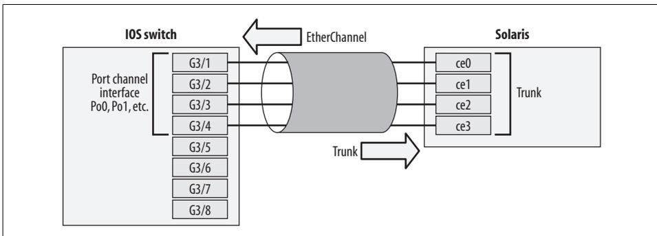
Figure 7-2. Cisco and Solaris terminology regarding EtherChannels
