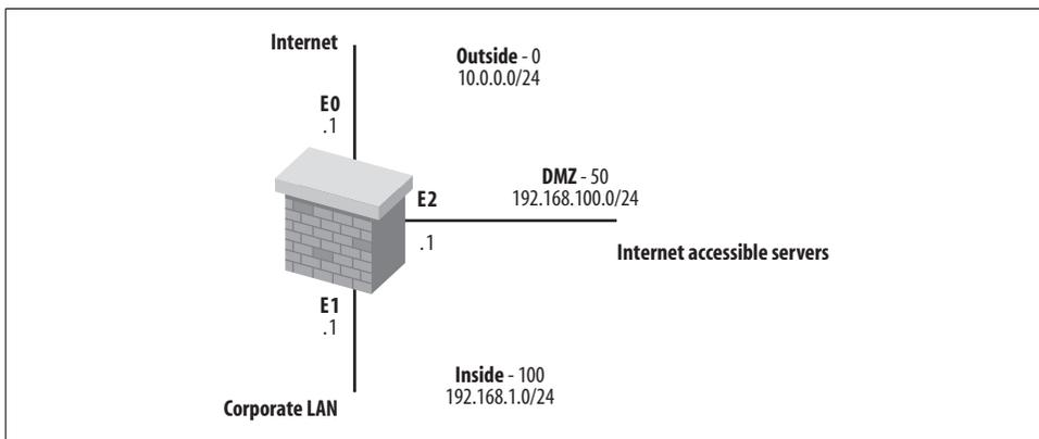
Figure 26-5. Firewall with DMZ
