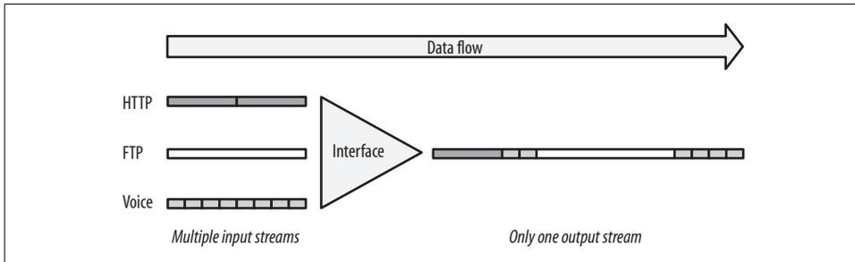
Figure 29-3. Packets through a serial interface
