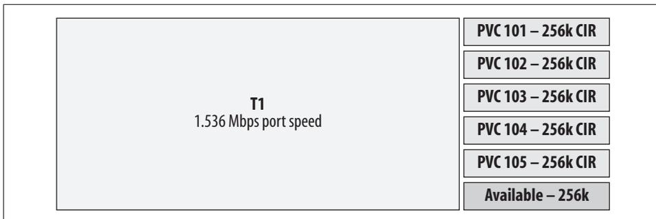
Figure 22-8. Subscription of a T1 using frame-relay PVCs
