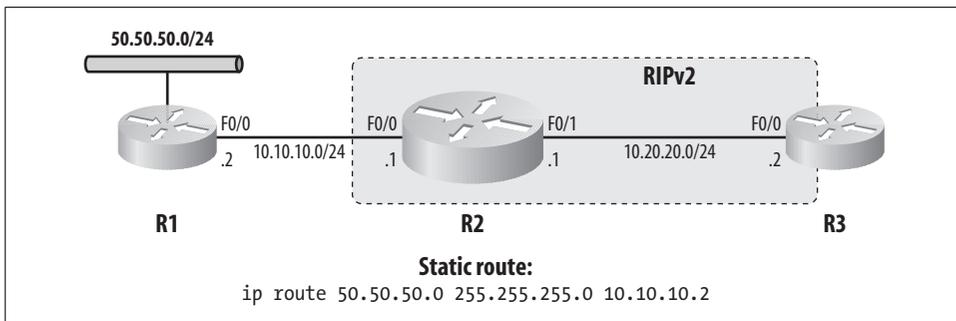
Figure 11-2. Redistributing a static route into RIPv2
