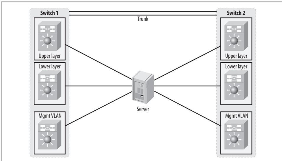
Figure 33-16. Ethernet interfaces in use on a server
