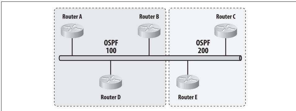
Figure 10-2. Two OSPF processes on a single network
