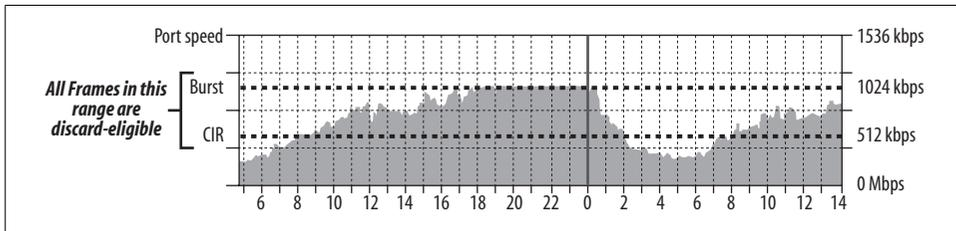
Figure 22-4. Frame-relay CIR and DE frames
