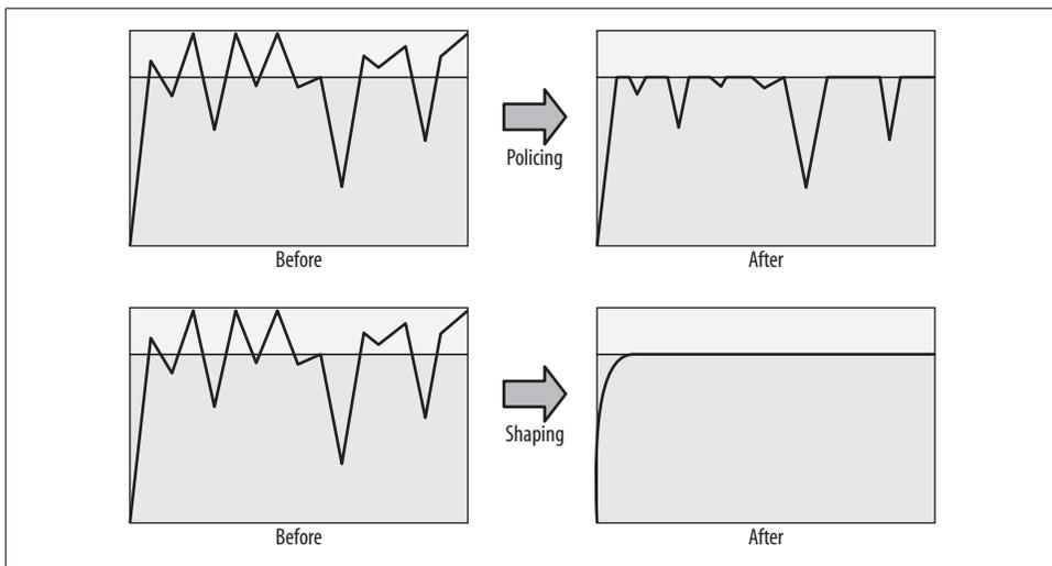
Figure 29-7. Traffic policing versus traffic shaping
