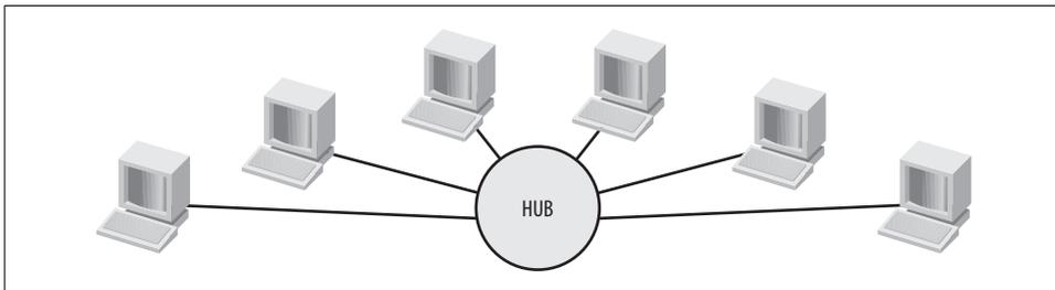
Figure 2-2. Hub connecting multiple hosts to a network
