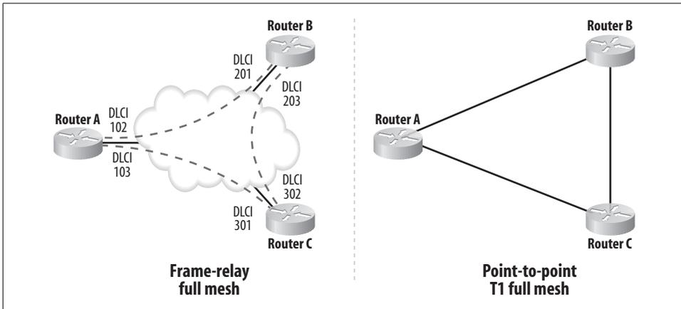
Figure 22-6. Frame-relay versus point-to-point T1 meshed networks
