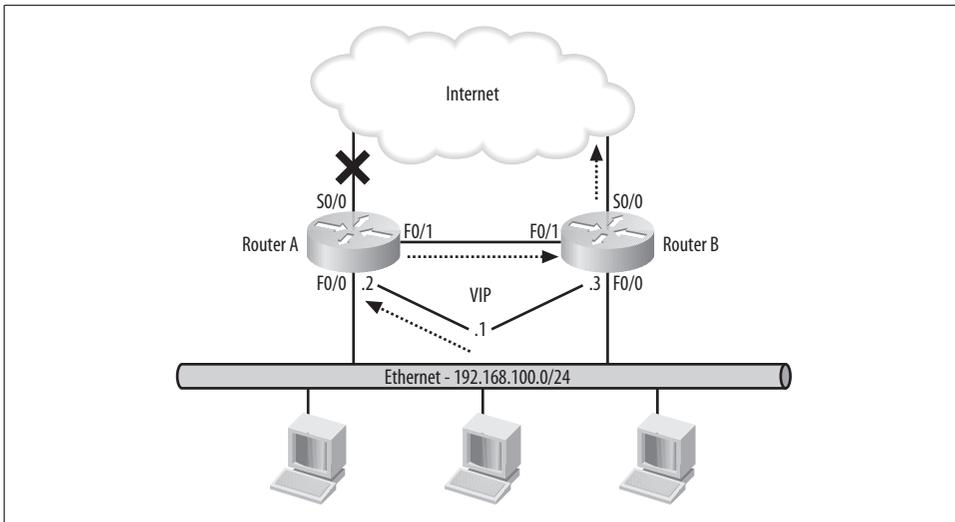
Figure 13-3. Primary Internet link failure without interface tracking
