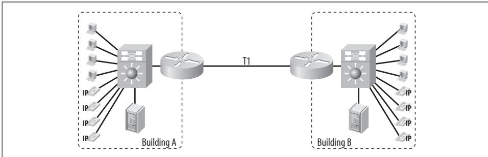
Figure 30-1. Two-building network with a single T1
