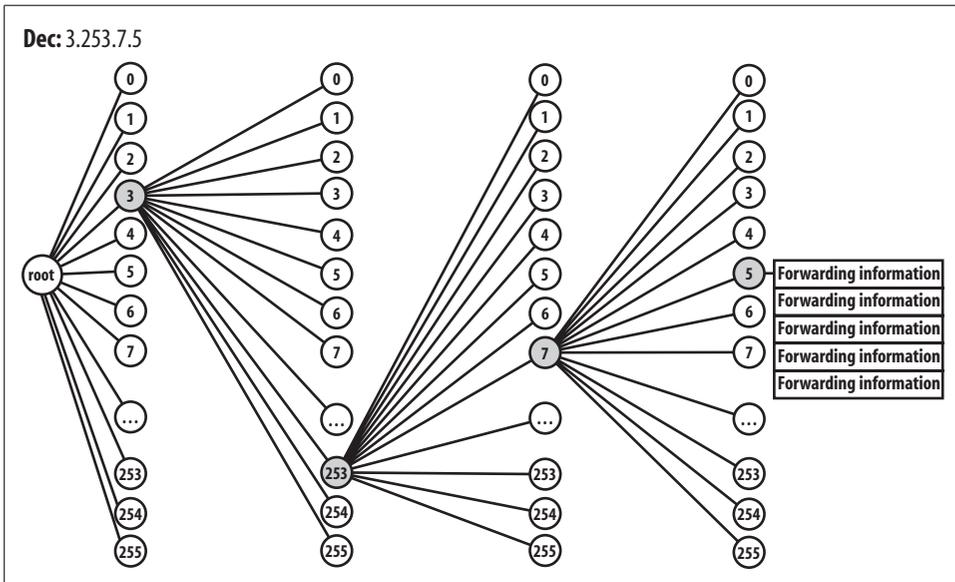
Figure 15-6. Data stored in optimum-switching multiway tree
