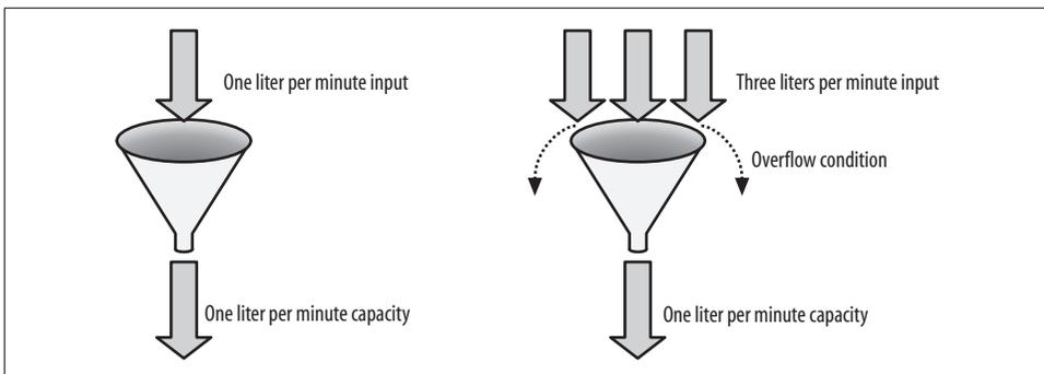
Figure 29-2. Overflow condition
