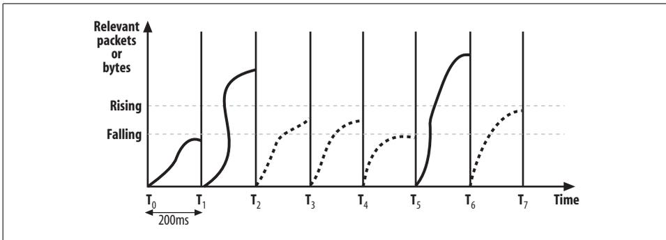
Figure 18-3. Rising and falling thresholds
