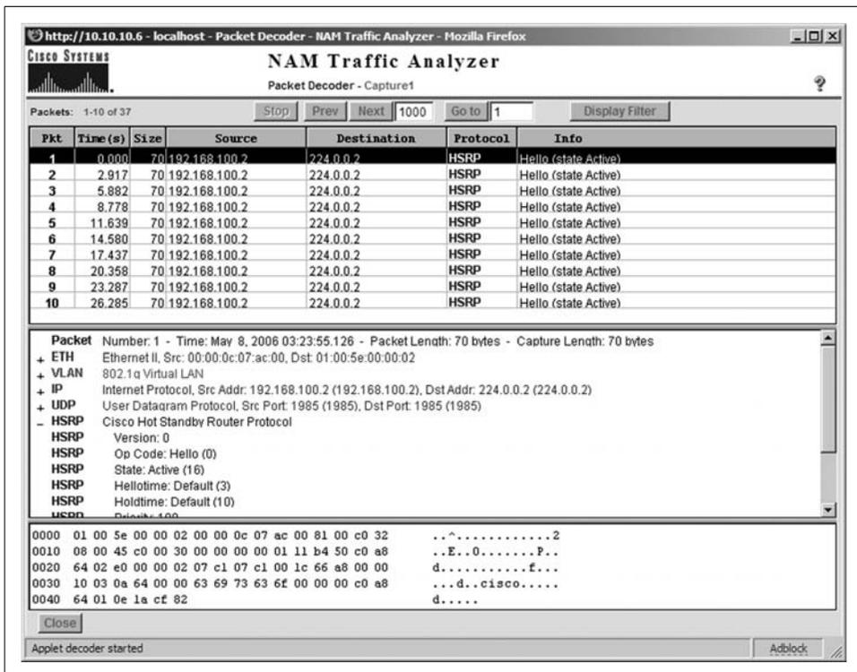
Figure 17-7. Network Analysis Module packet capture detail
