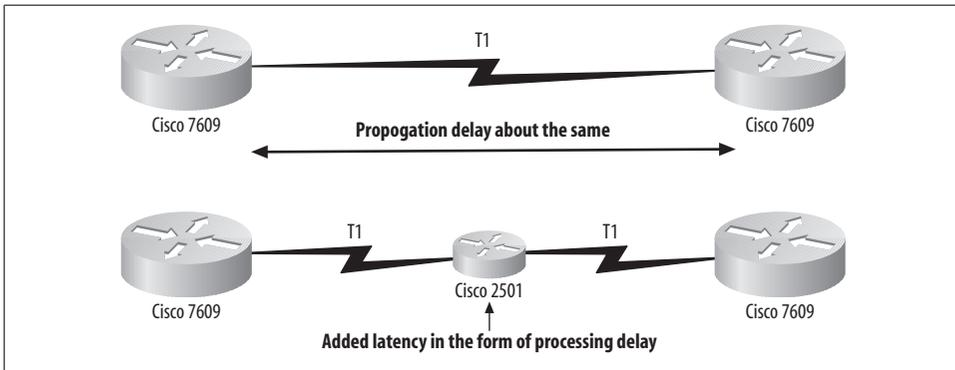
Figure 19-5. Processing delay
