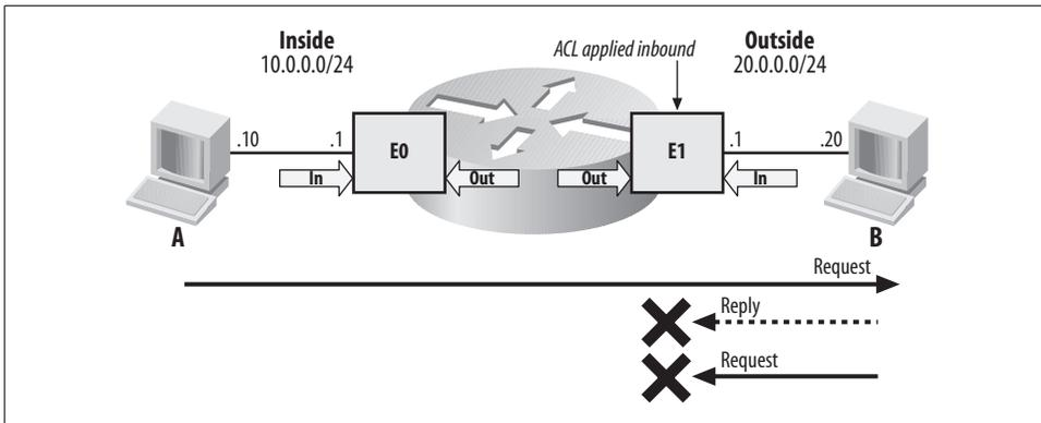
Figure 23-4. Simple access list applied inbound on E1
