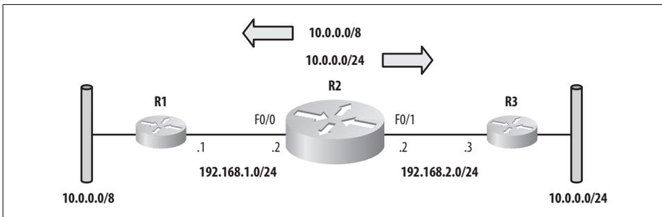
Figure 9-1. Same network with different prefix lengths
