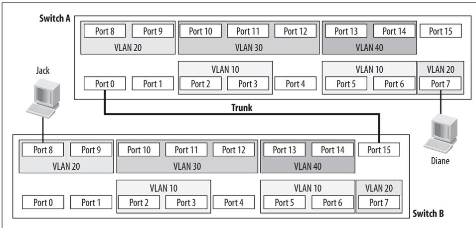
Figure 4-3. Two switches connected with a trunk
