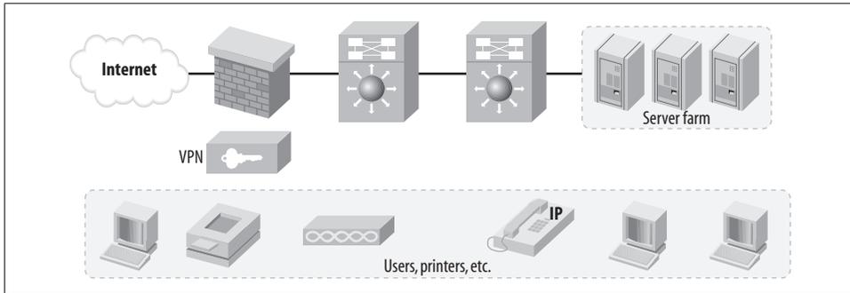
Figure 33-11. Collapsed-core network consisting of only one layer
