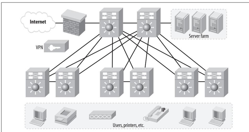
Figure 33-10. Collapsed-core network without a distribution layer
