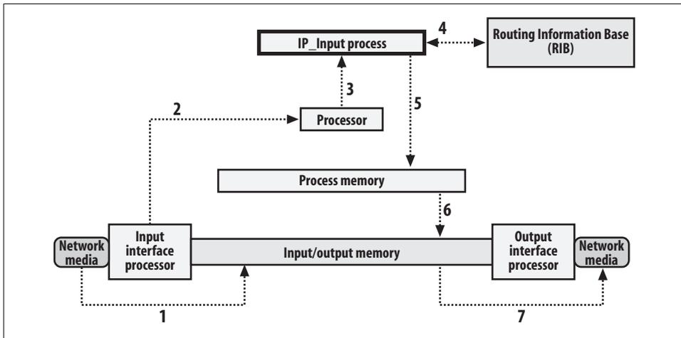
Figure 15-2. Process switching
