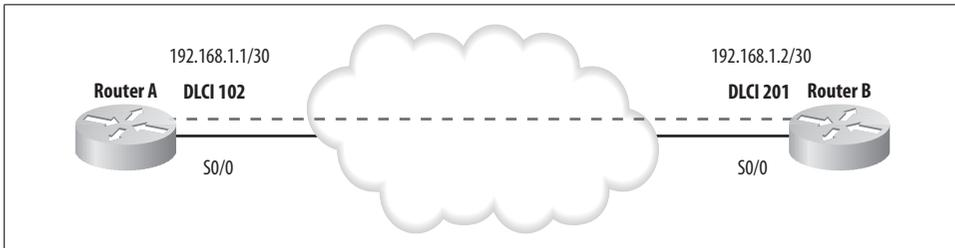
Figure 22-10. Two-node frame-relay network
