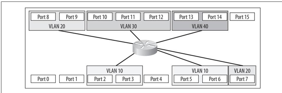
Figure 16-1. VLANs routed from within a switch
