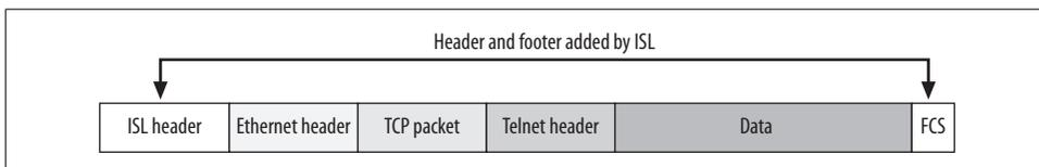
Figure 5-3. ISL encapsulated frame
