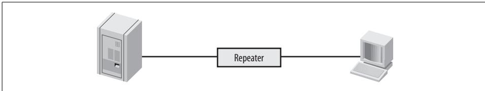
Figure 2-1. Repeater extending a single 10Base-T link
