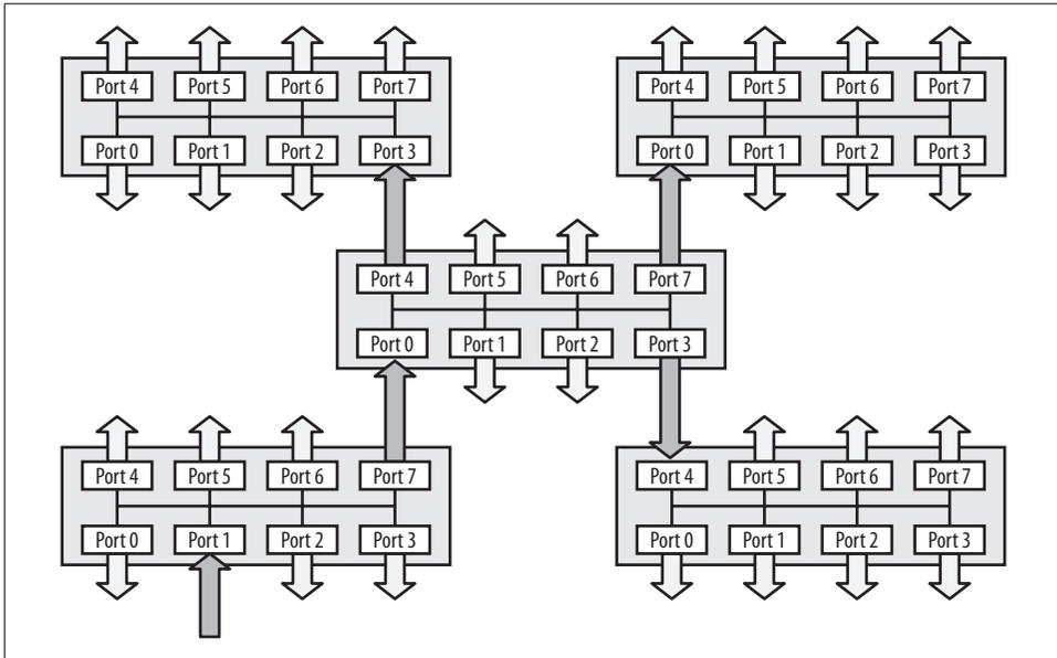
Figure 2-5. Hub-based network
