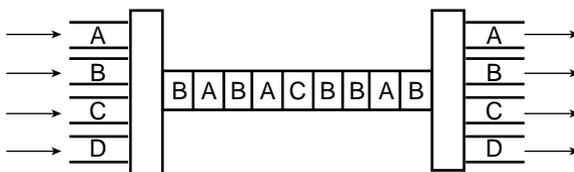
**FIGURE 3.6** Statistical time-division multiplexing allocates timeslots based on a channel's traffic demand.
