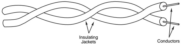
Twisting of the wires also controls the tendency of the wires in the pair to cause EMI in each other. As noted previously, whenever two wires are in close proximity, the signals in each wire tend to produce crosstalk in the other. Twisting the wires in the pair reduces crosstalk in much the same way that twisting reduces the tendency of the wires to radiate EMI.
