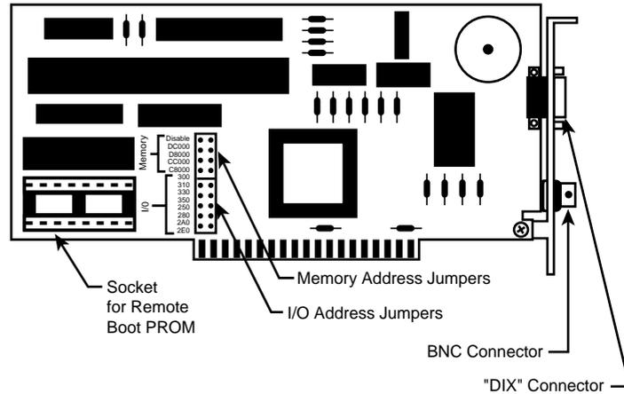
Network adapter cards play an important role on the network. They are responsible for translating data from a device on the network—mostly computers—and converting this data into some form of signal that can be transmitted across the transmission medium. To enable you to understand the full functionality of the network adapter card, the specific functions of what the network card does must each be addressed.
