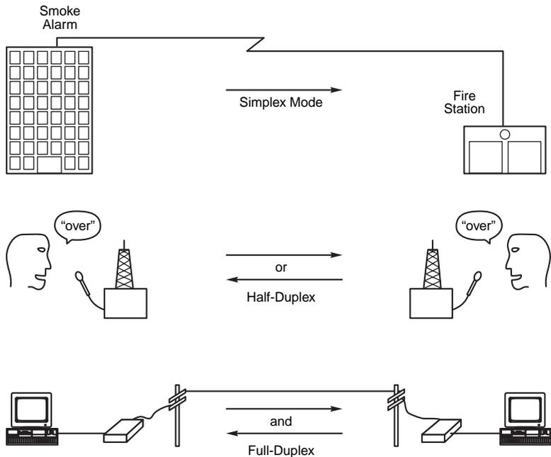
Half-duplex communication can result in wasted bandwidth during the intervals when communication is turned around. On the other hand, using full-duplex communication generally requires a greater bandwidth than half-duplex communication.
