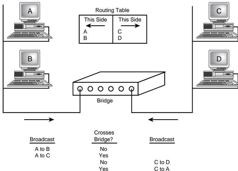
**FIGURE 2.5** Bridges isolate traffic on a single network segment.
