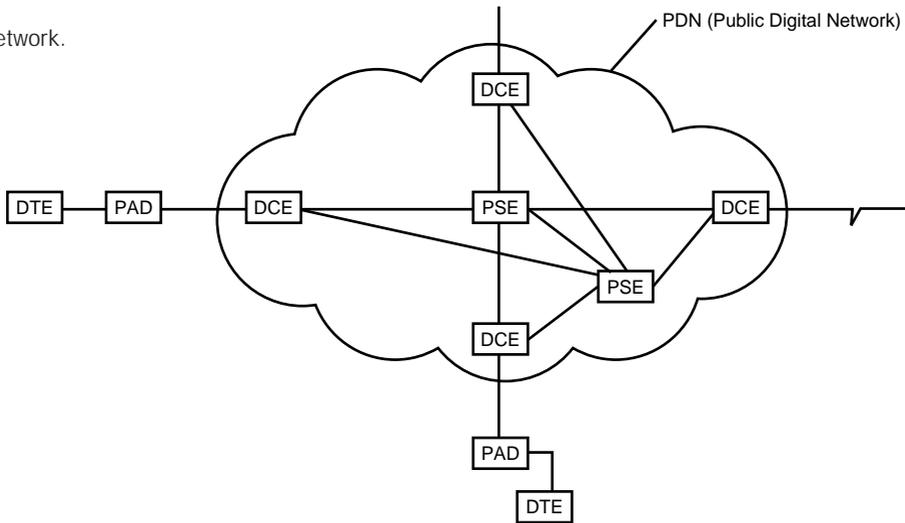
The X.25 protocol oversees the communication between the DTE and the DCE. A device called a *packet assembler/disassembler (PAD)* translates asynchronous input from the DTE into packets suitable for the PDN.
