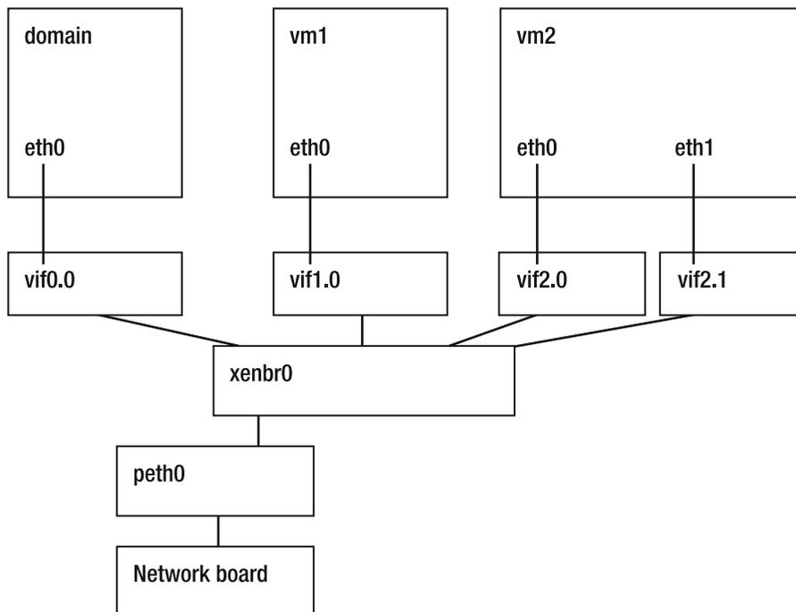
**Figure 13-7.** *The virtual bridge in a Xen environment*
