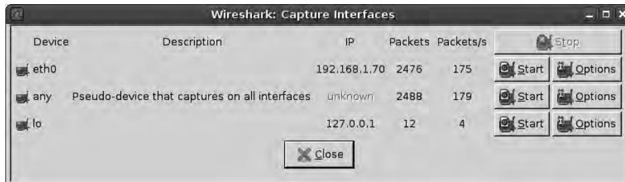
**Figure 8-4.** Before starting a Wireshark packet capture, select the interface you want to perform the packet capture on and then click **Start**.
