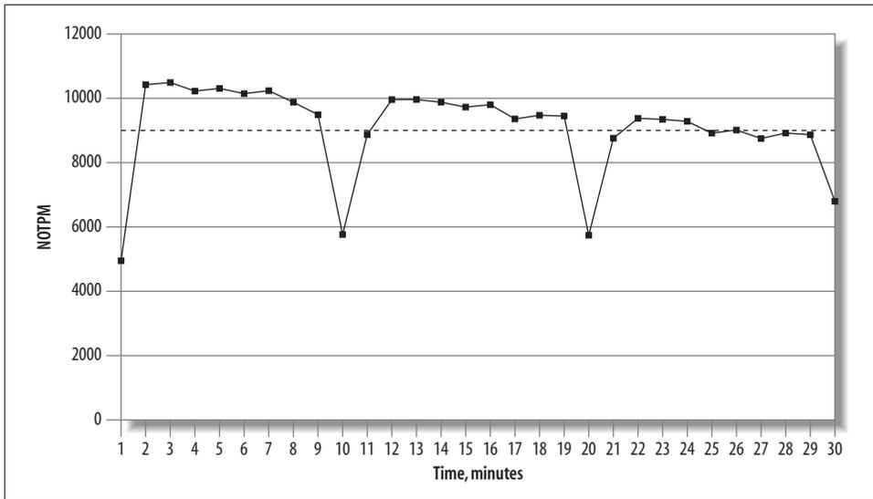
Figure 2-1. Results from a 30-minute dbt2 benchmark run
