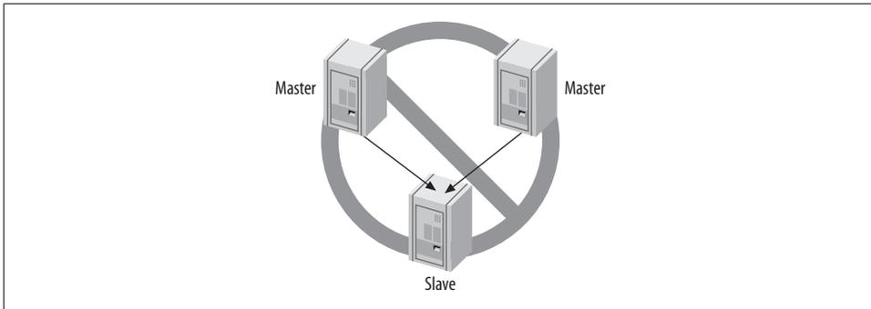
Figure 8-6. MySQL does not support multimaster replication
