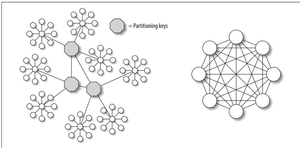
Figure 9-4. Two data models, one easy to shard and the other difficult<sup>a</sup>
