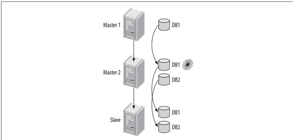
Figure 8-14. Another way to emulate multimaster replication
