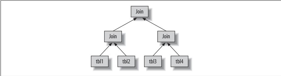
Figure 4-3. One way to join multiple tables
